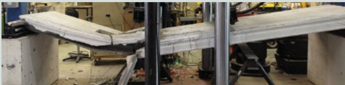
Slab SO-S at failure
