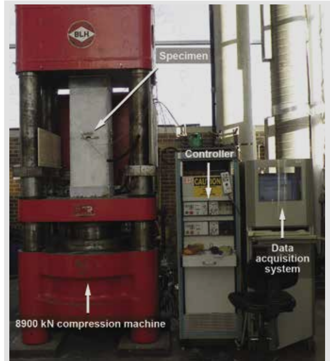
Figure 7. Test setup for short pile specimens.
