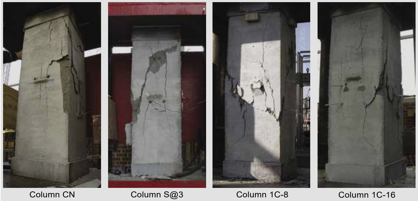
Figure 10. Short test piles at the conclusion of the test.
