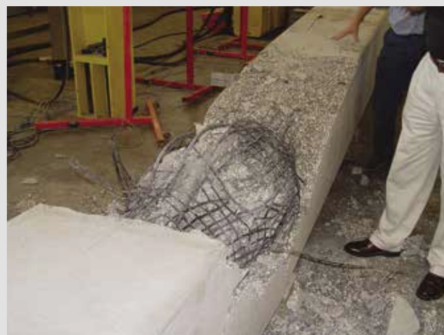
Figure 20. Failure of pile with carbon-fiber-reinforced polymer grid due to concrete crushing.
