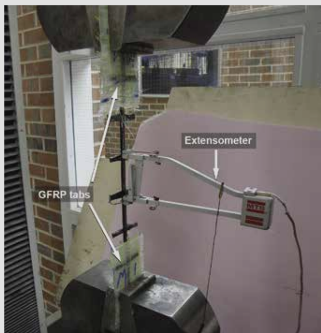
Figure 1. Testing of carbon-fiber-reinforced polymer grid tension coupon. Note: GFRP = glass-fiber-reinforced polymer.
