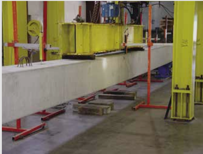
Figure 17. Pile with carbon-fiber-reinforced polymer grid before testing.
