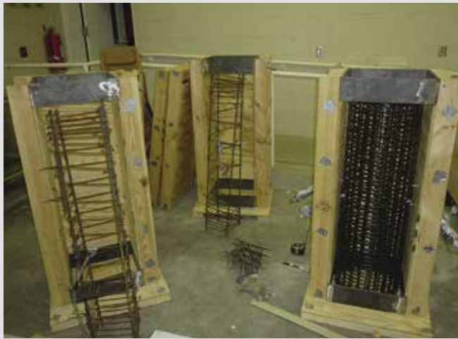
Figure 6. Short column specimens with steel spirals or carbon-fiber-reinforced polymer grids in wooden forms.
