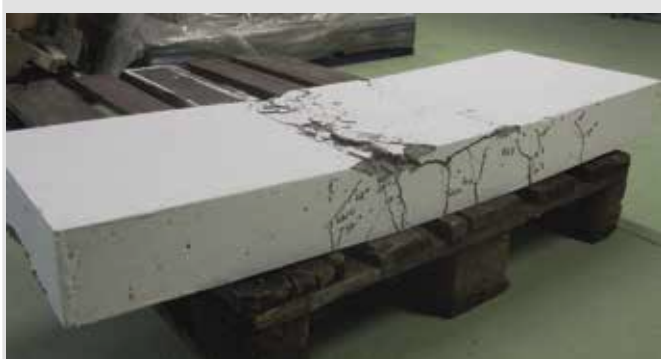
Figure 5. Failure mode of the panels reinforced with basalt-fiber-reinforced polymer.
