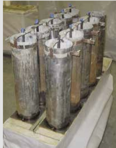
Figure 1. ASTM A1081 specimens before mortar placement.
