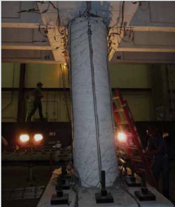
Column at 7 in. lateral displacement (displacement ductility +10.0)
