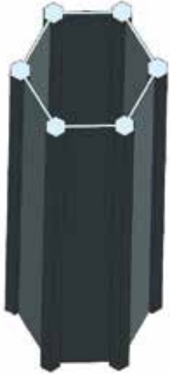
Figure 2. A schematic view of a Hexcrete tower section.
