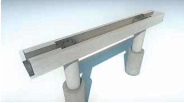
The seismic-resistant intermediate piers comprise precast concrete columns and partially precast concrete crossbeams. Connections developed as part of the Highways for Life program were used to connect the columns and crossbeams. The crossbeams were partially precast to limit their pick weight. Courtesy of Greg Banks.
