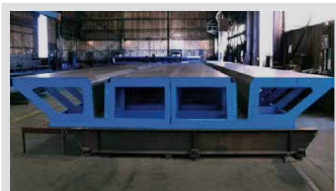
Figure 12. Split 16 ft wide double-tee form. Note: 1 ft = 0.305 m. Courtesy of Hamilton Form.
