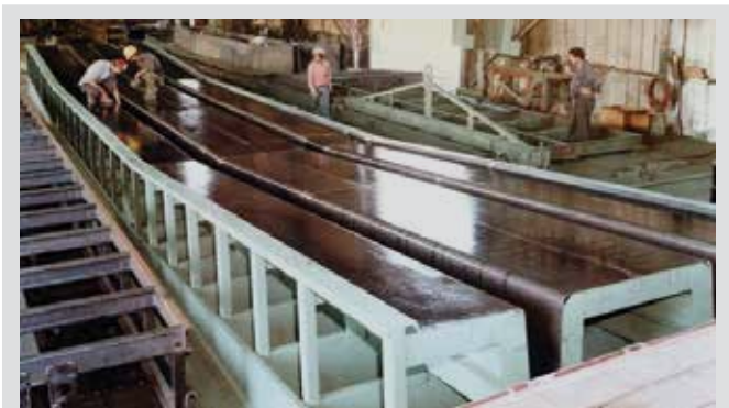
Figure 21. Concave formwork for parking ramp double tee. Courtesy of Hamilton Form.
