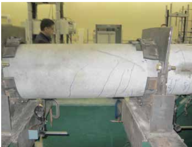
Figure 7. Shear cracks between supports prior to failure.
