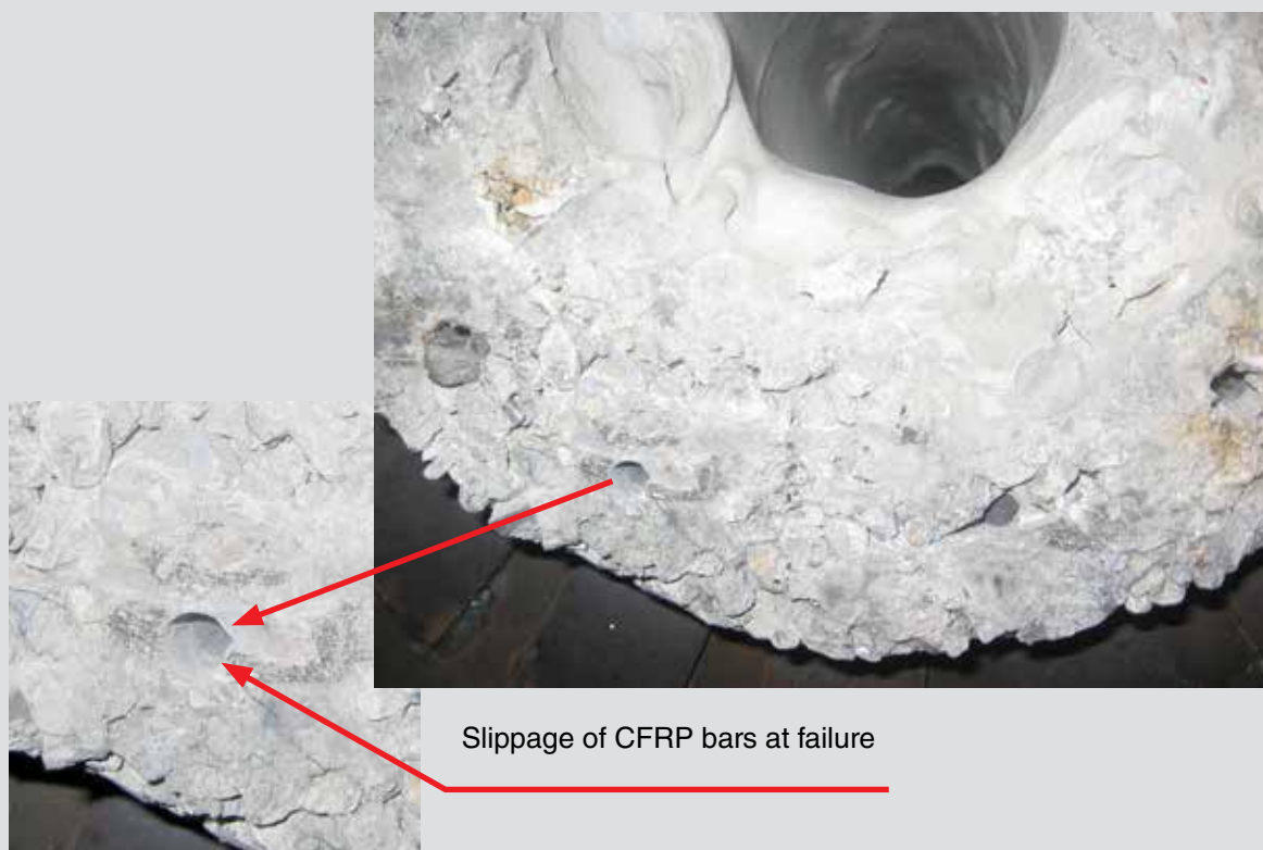
Figure 11. Slippage of CFRP bars at failure of poles confined with CFRP grid. Note: CFRP = carbon-fiber-reinforced polymer.
