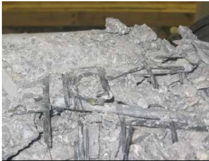
Figure 10. Rupture of carbon-fiber-reinforced polymer grid used for pole confinement.
