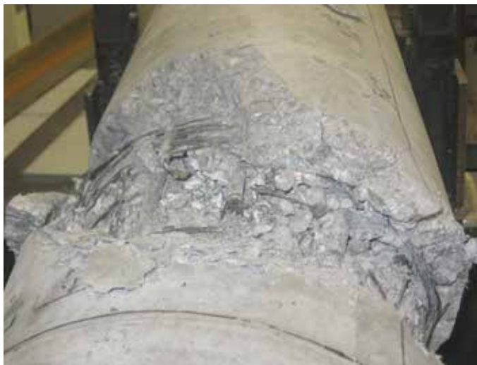
Figure 9. Breaking of carbon-fiber-reinforced polymer (CFRP) bars for poles confined with CFRP grid.
