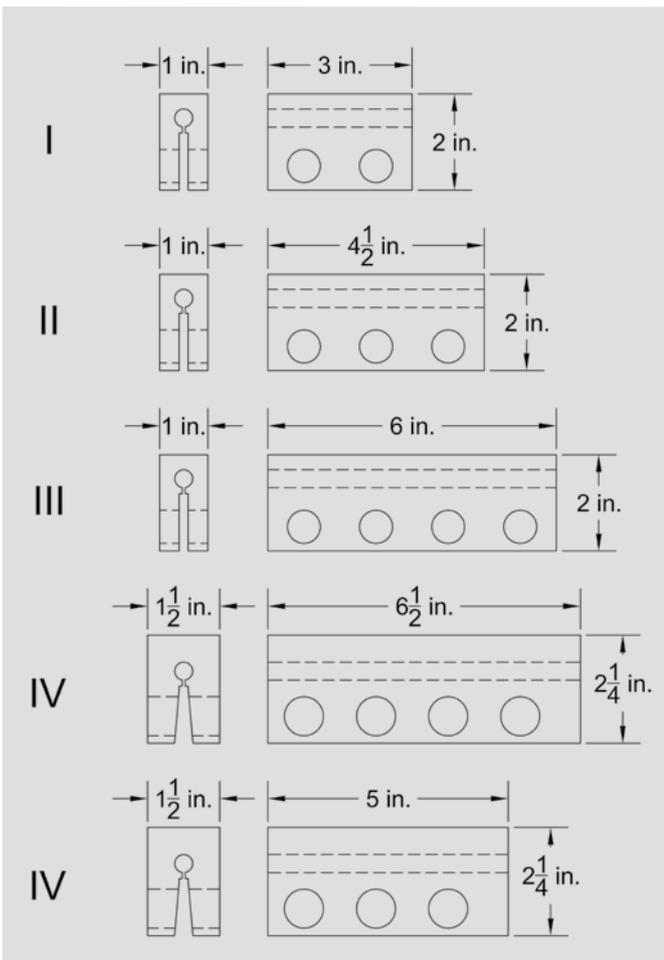
**Figure 2.** Anchor size comparison across generations I-III, IV four-bolt, and IV three-bolt anchors. Note: 1 in. = 25.4 mm.
