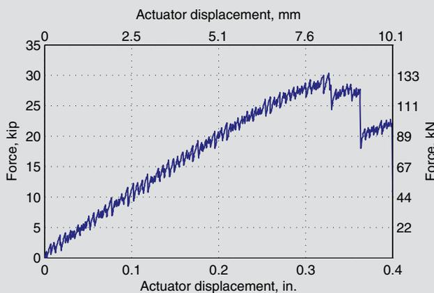
**Applied force versus actuator displacement**
