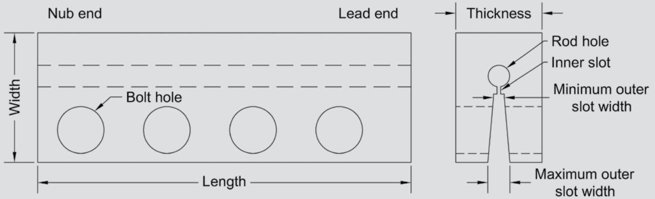
**Figure 1.** Unibody clamp anchor geometry.
