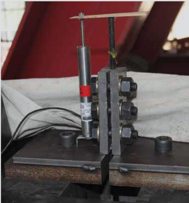
**Linear variable differential transducer setup**
