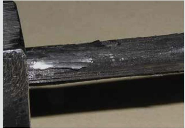
**Damage caused to CFRP rod from slip**
