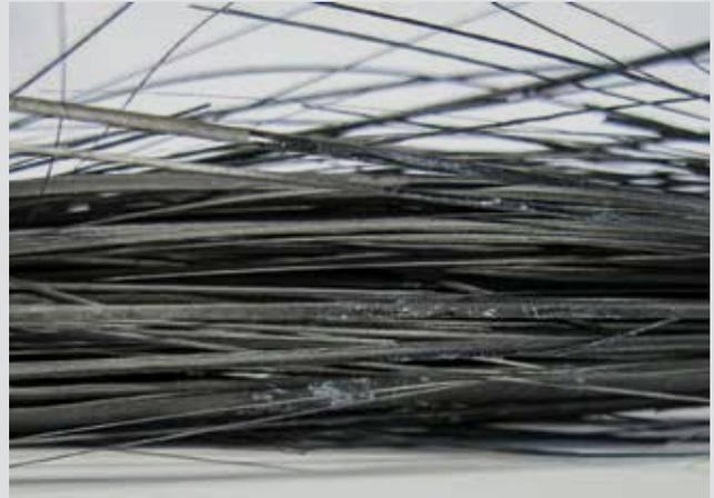
**CFRP rod tensile failure**
