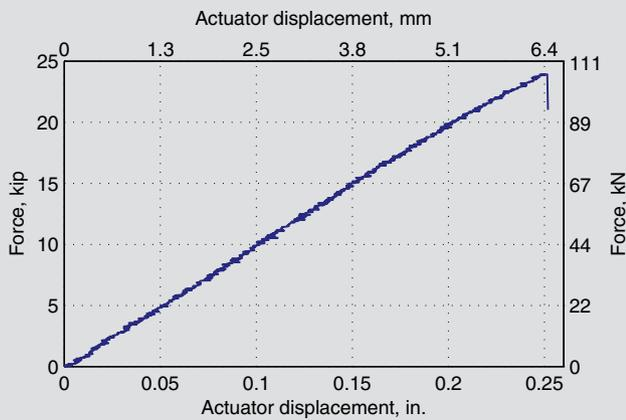
**Applied force versus actuator displacement**
