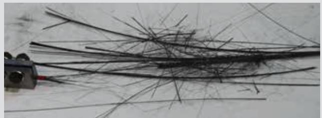
**Tensile failure of CFRP rod**
