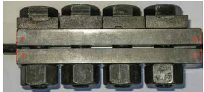
**Figure 10.** Clamped generation IV anchor showing increased width of outer slot from nub to lead end (A-A to B-B).
