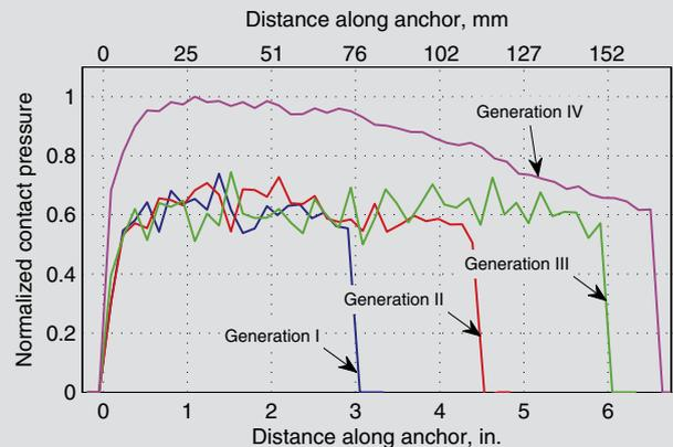
**Normalized contact pressure on side of carbon-fiber-reinforced polymer rod for generations I through IV (0 in. [0 mm] = nub end, 6.5 in. [165 mm] = lead end)**
