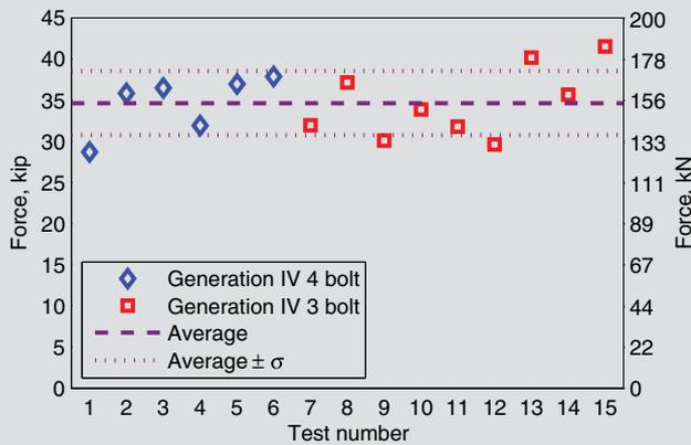
**Figure 12.** Distribution of generation IV test results for three-bolt and four-bolt anchors. Note:  $\sigma$  = standard deviation.
