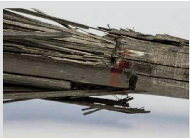
**Ruptured CFRP rod located at lead edge**
