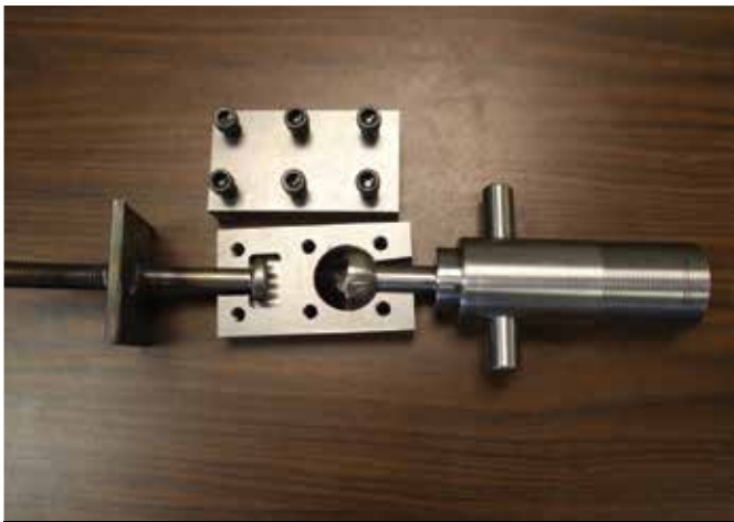
Figure 3. Stud assembly loaded in the Instron.
