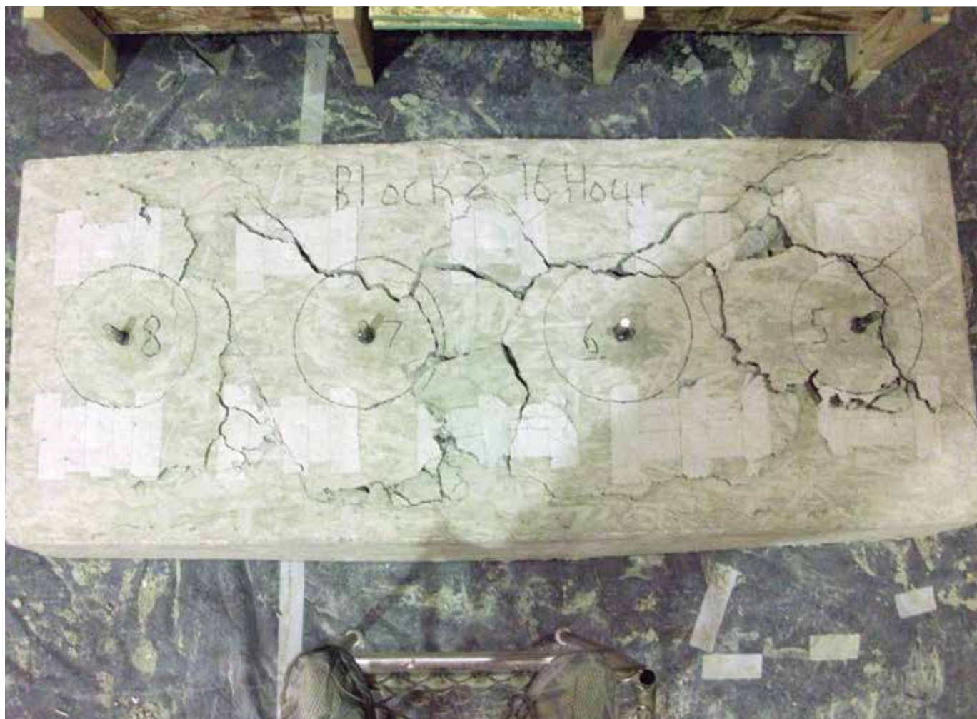
Figure 6. Typical breakout failure pattern at 16 hours.
