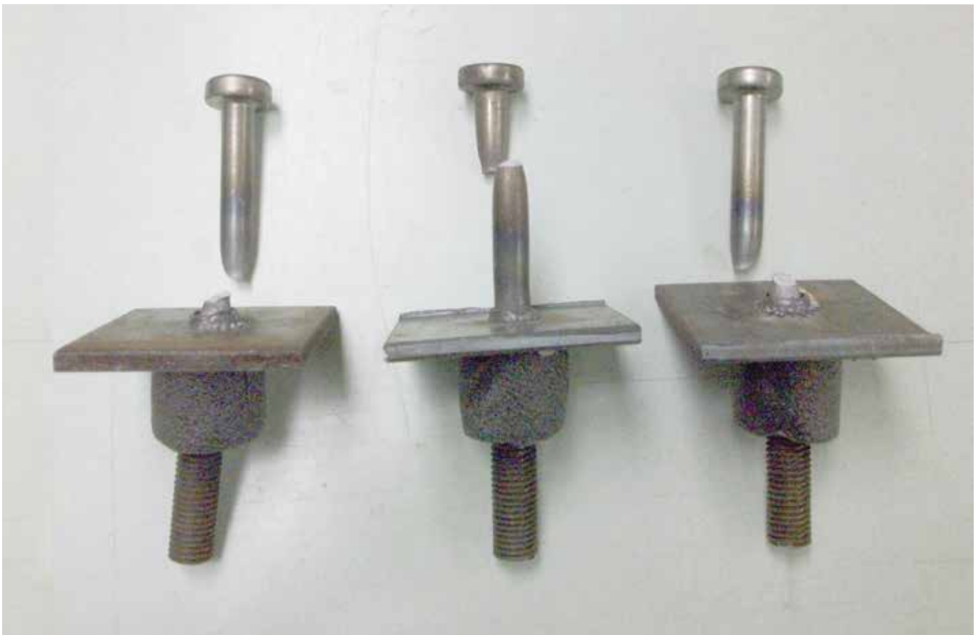
Figure 11. Headed studs after testing.
