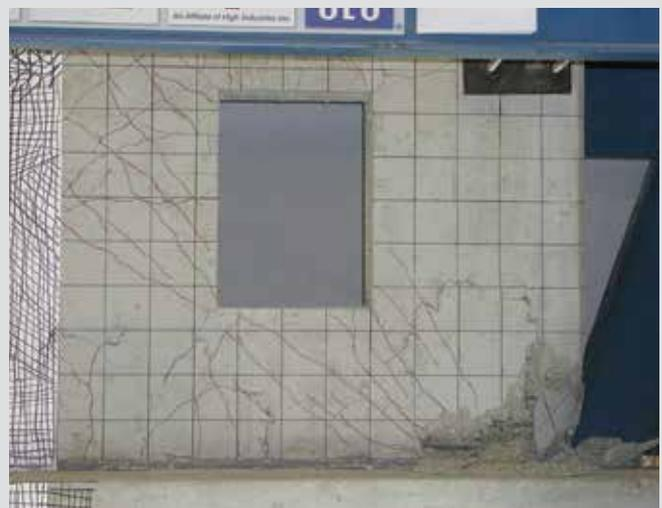
**Figure 5.** Performance of base panel north toe. Note: 1 mm = 0.0394 in.
