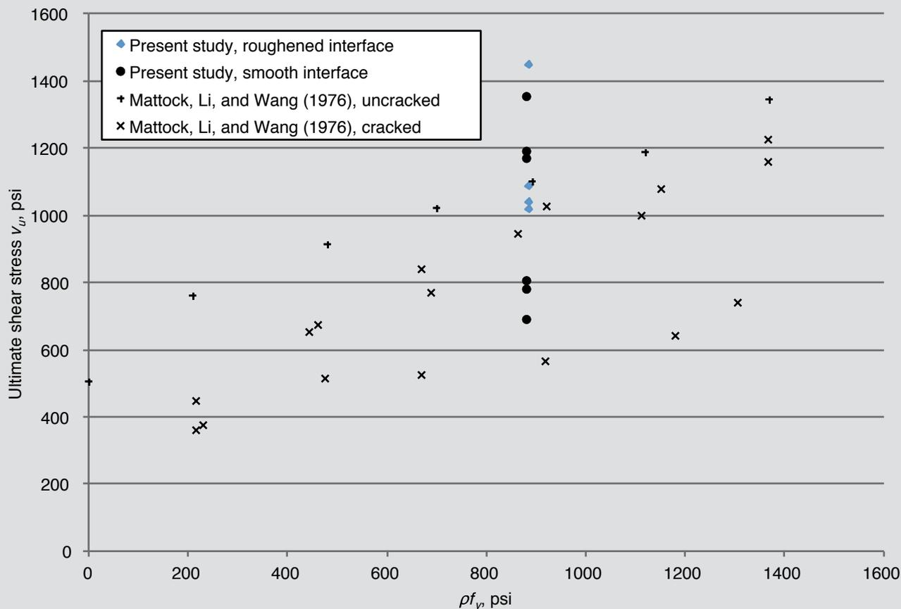
**Figure 10.** Comparison of ultimate shear stress  $v_u$  for specimens with different interface conditions for sand-lightweight concrete. Note:  $f_y$  = yield stress of reinforcement;  $\rho$  = shear friction reinforcement ratio. 1 psi = 6.895 kPa.
