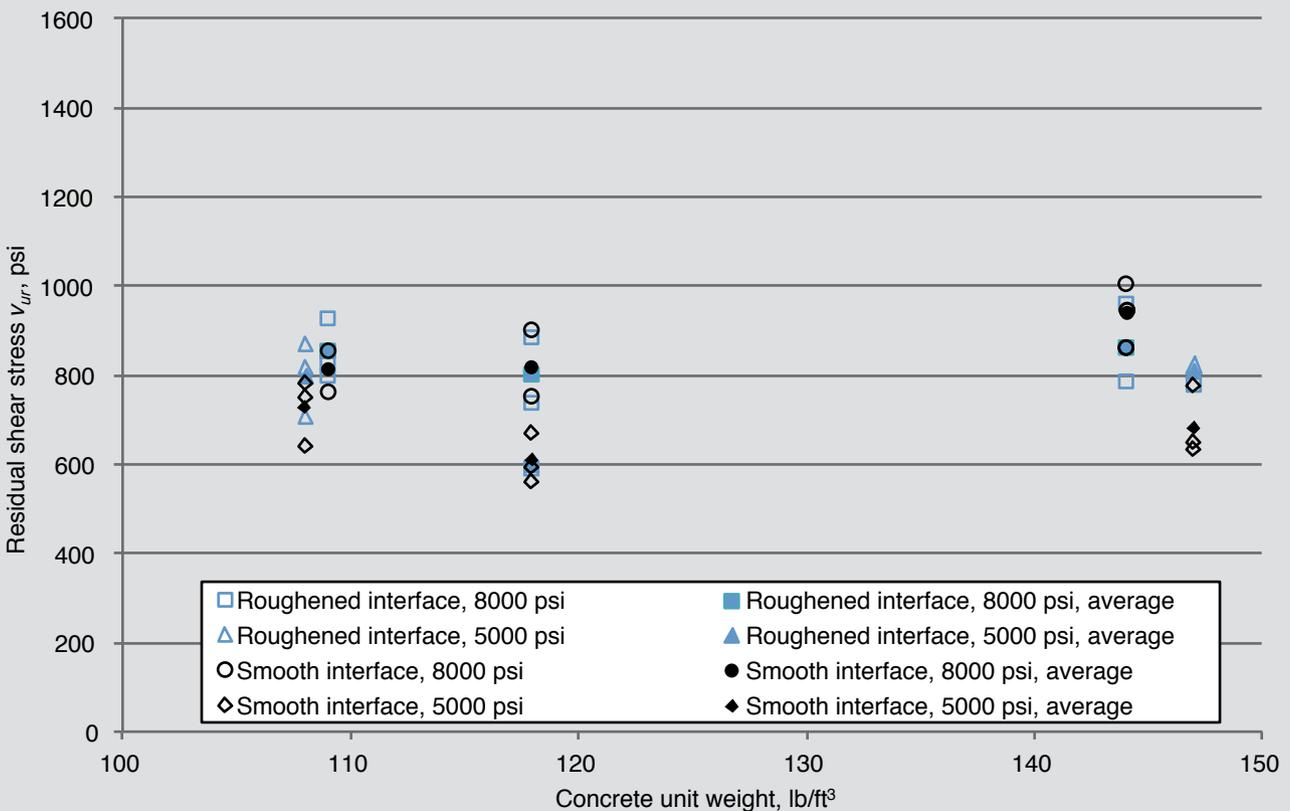
**Figure 9.** Comparison of residual shear stress  $v_{ur}$  versus concrete unit weight. Note: 1 ft = 0.305 m; 1 lb = 0.454 kg; 1 psi = 6.895 kPa.
