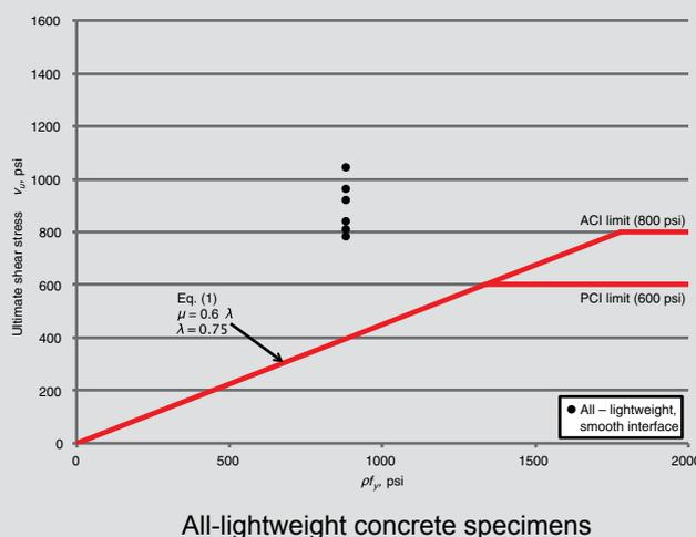
**Figure 13.** Comparison of ultimate shear stress  $v_u$  with Eq. (1) for specimens with a smooth interface. Note:  $f_y$  = yield stress of reinforcement;  $\lambda$  = modification factor reflecting the reduced mechanical properties of lightweight concrete relative to normalweight concrete of the same compressive strength;  $\mu$  = coefficient of friction;  $\rho$  = shear friction reinforcement ratio. 1 psi = 6.895 kPa.
