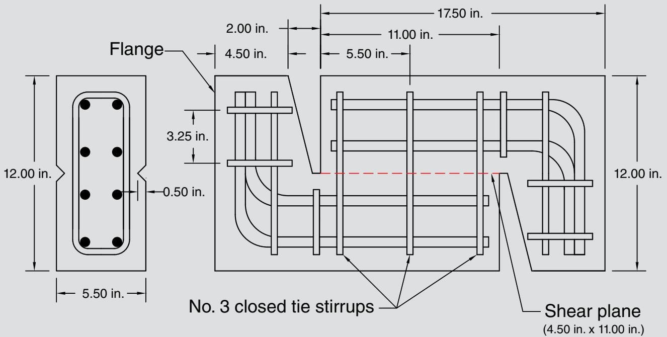
**Figure 2.** Test specimen. Note: dimensions shown in figure are measured to nearest 0.25 in. No. 3 = 10M; 1 in. = 25.4 mm.
