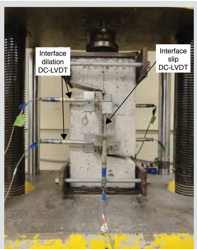
**Figure 4.** Test setup and instrumentation. Note: DC-LVDT = direct current linear variable displacement transducer.
