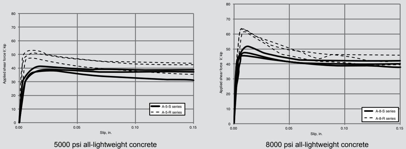
**Figure 7.** Applied shear force  $V$ –slip relations for all-lightweight concrete specimens. Note: 1 in. = 25.4 mm; 1 kip = 4.448 kN; 1 psi = 6.895 kPa.
