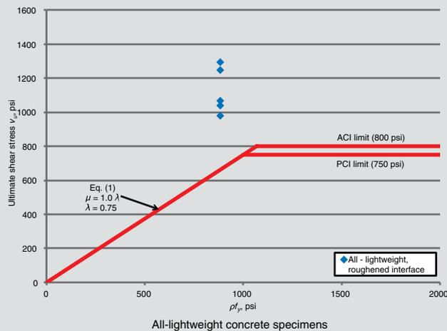
**Figure 12.** Comparison of ultimate shear stress  $v_u$  with Eq. (1) for specimens with a roughened interface. Note:  $f_y$  = yield stress of reinforcement;  $\lambda$  = modification factor reflecting the reduced mechanical properties of lightweight concrete relative to normalweight concrete of the same compressive strength;  $\mu$  = coefficient of friction;  $\rho$  = shear friction reinforcement ratio. 1 psi = 6.895 kPa.
