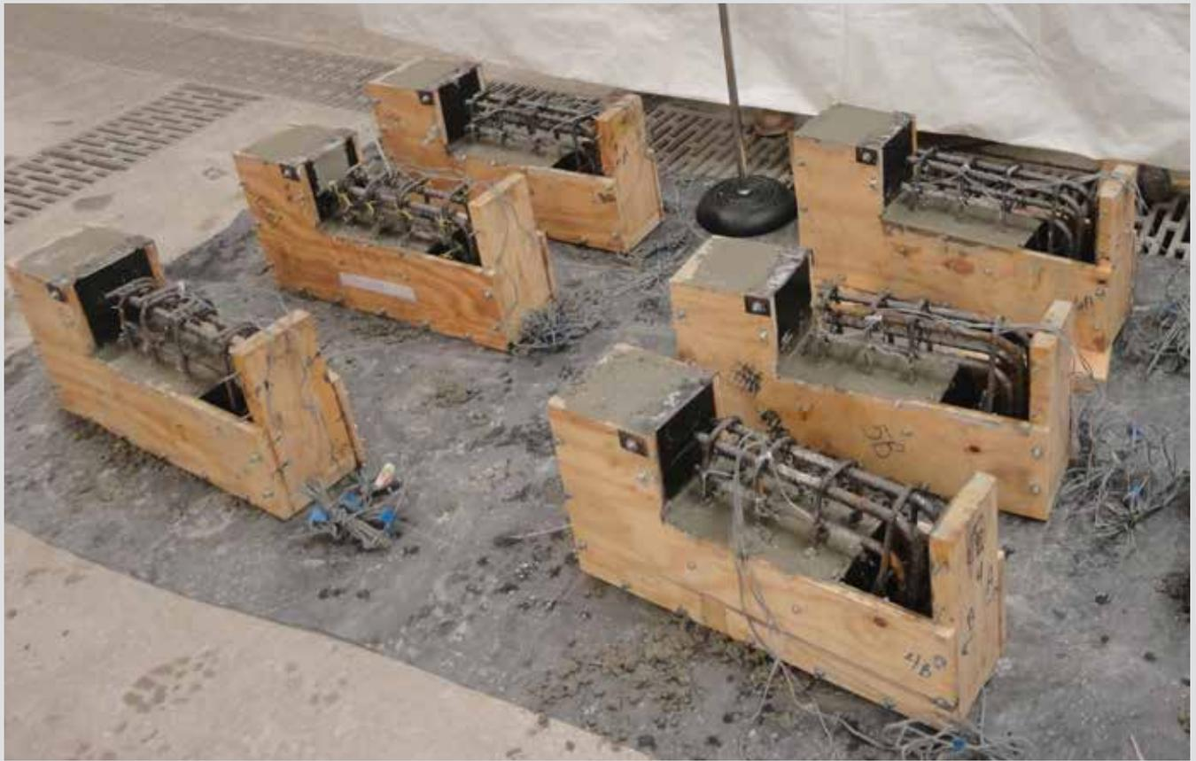
**Figure 3.** Test specimen casting.
