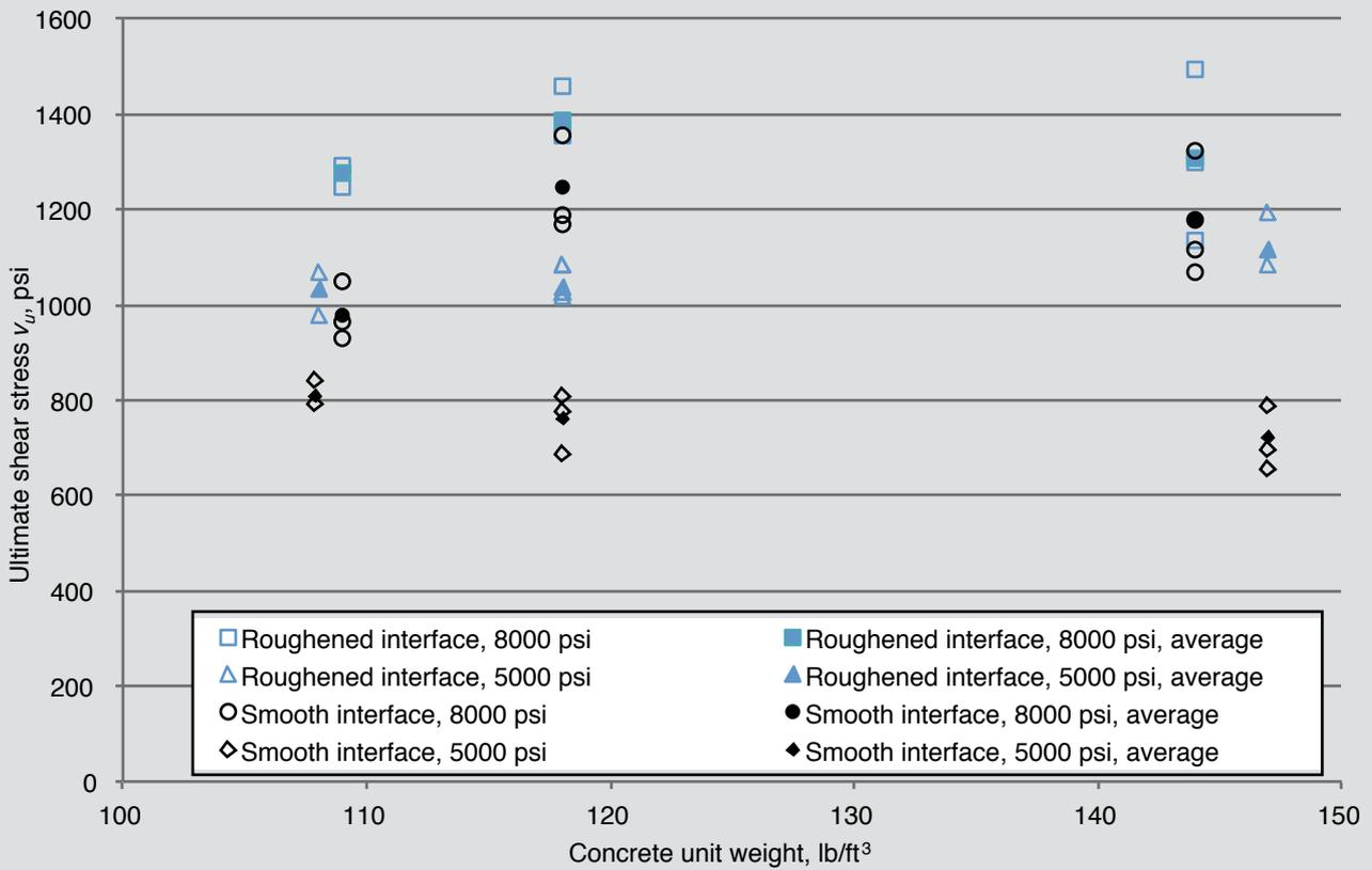
**Figure 8.** Comparison of ultimate shear stress  $v_u$  versus concrete unit weight. Note: 1 ft = 0.305 m; 1 lb = 0.454 kg; 1 psi = 6.895 kPa.
