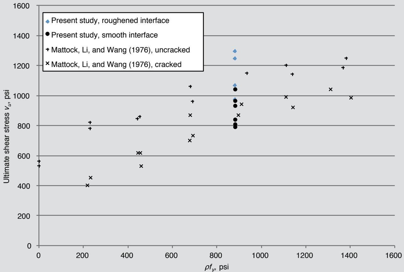
**Figure 11.** Comparison of ultimate shear stress  $v_u$  for specimens with different interface conditions for all-lightweight concrete. Note:  $f_y$  = yield stress of reinforcement;  $\rho$  = shear friction reinforcement ratio. 1 psi = 6.895 kPa.
