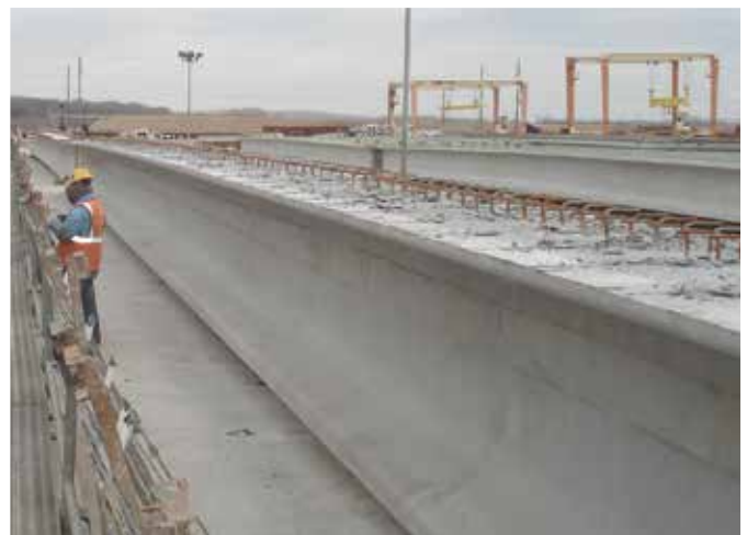
Figure 8. Camber of 140 ft (43 m) girders at release.
