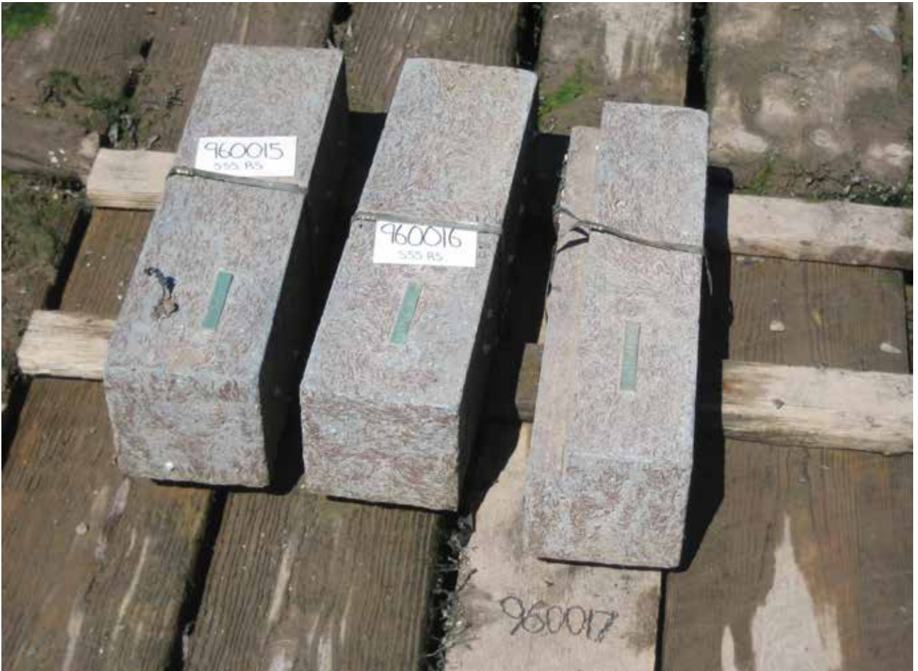
Figure 7. Test prisms on the wharf at a long-term exposure test site in Treat Island, Maine. Courtesy of Lafarge.
