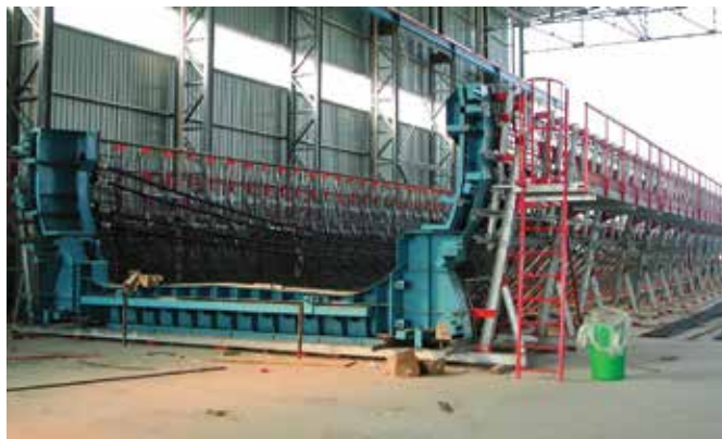
Figure 4. Reinforcing bar jig for full-span cage prefabrication of a single-track U beam.
