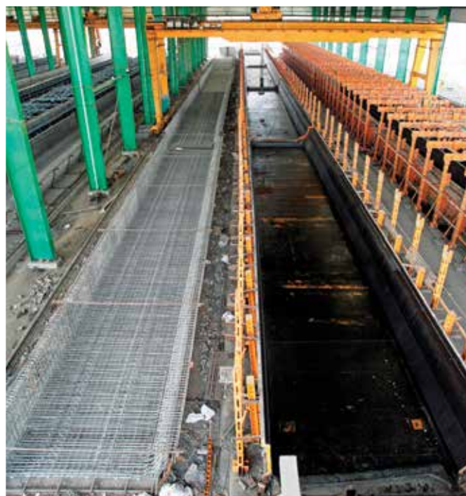
Figure 1. Four-bed casting line. Courtesy of Systra.
