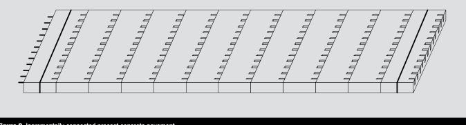
Figure 9. Incrementally connected precast concrete pavement.
