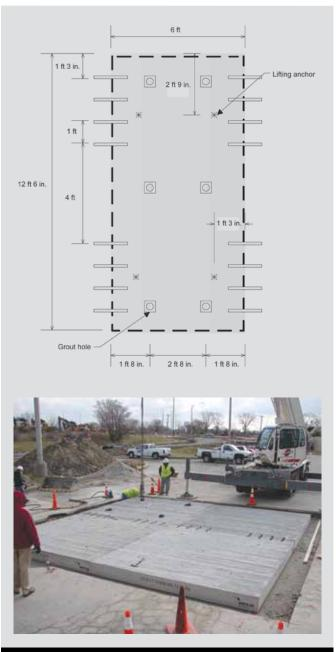
Figure 12. Illinois Tollway intermittent repair system. Note: 1 in. = 25.4 mm; 1 ft = 0.305 m.
