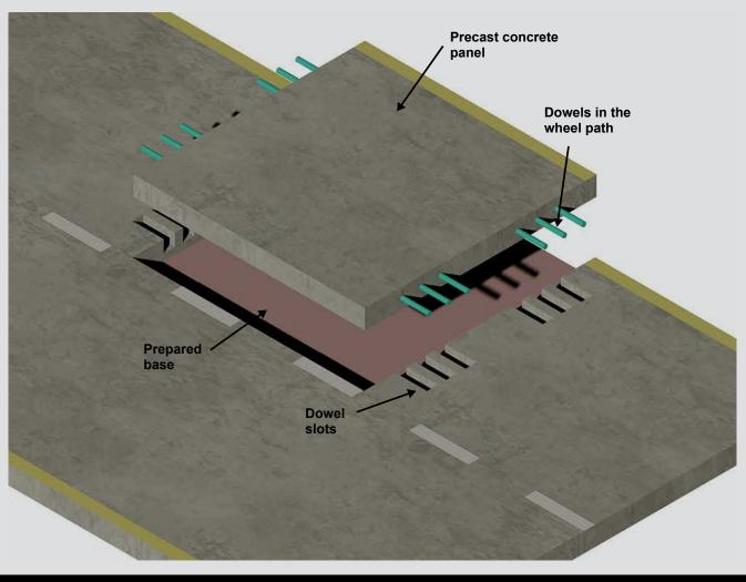
Figure 2. One scheme for intermittent repairs.
