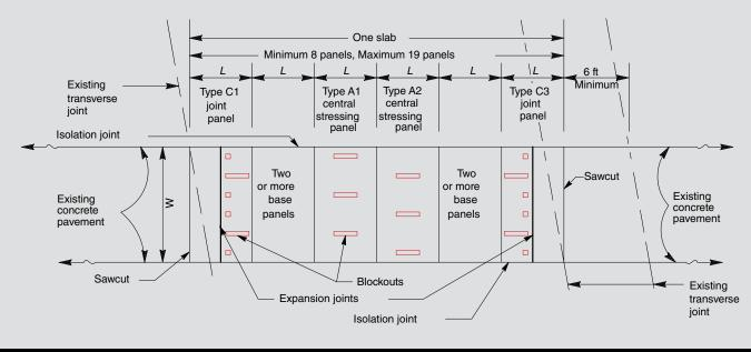
Figure 1. Original precast, posttensioned concrete pavement slab layout. Note: A slab is a series of panels L = length of panel. 1 ft = 0.305 m.
