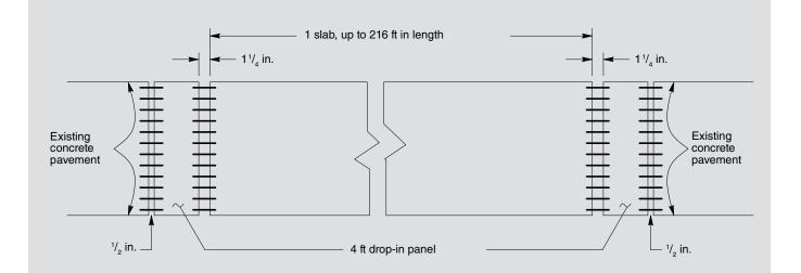
Figure 3. Modified precast, posttensioned concrete pavement layout and permanent 4 ft drop-in panel. Note: A slab is a series of panels. 1 in. = 25.4 in.; 1 ft = 0.305 m.
