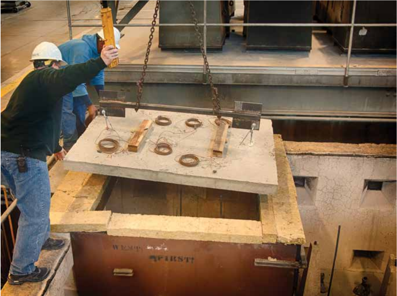
A basalt-fiber-reinforced-polymer reinforced precast concrete panel is lowered into position for testing for fire resistance in accordance with ASTM E119. New materials and construction methods that differ from the standard prescriptive assemblies must be tested to demonstrate compliance with the International Building Code . Courtesy of Paul Grigonis.
