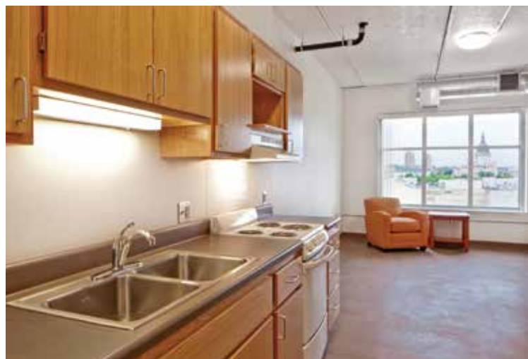
An efficiency apartment on the seventh floor of the Higher Ground homeless shelter has kitchen facilities and its own bathroom. The ceilings are formed by painted hollow-core units; no additional finishes were necessary. Residents can use their Catholic Charities cards to buy fresh food in season at the nearby Minneapolis Farmer's Market. They get the best deals on produce shortly before the market closes for the day. Photograph by Brandon Stengel. Courtesy of Hanson Structural Precast.
