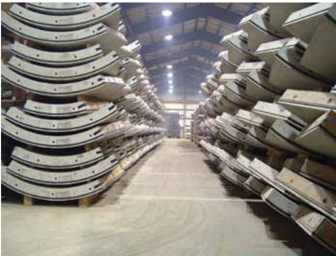
Figure 13. Segmental tunnel lining using steel-fiber-reinforced concrete. Courtesy of Bekaert Corp. USA.
