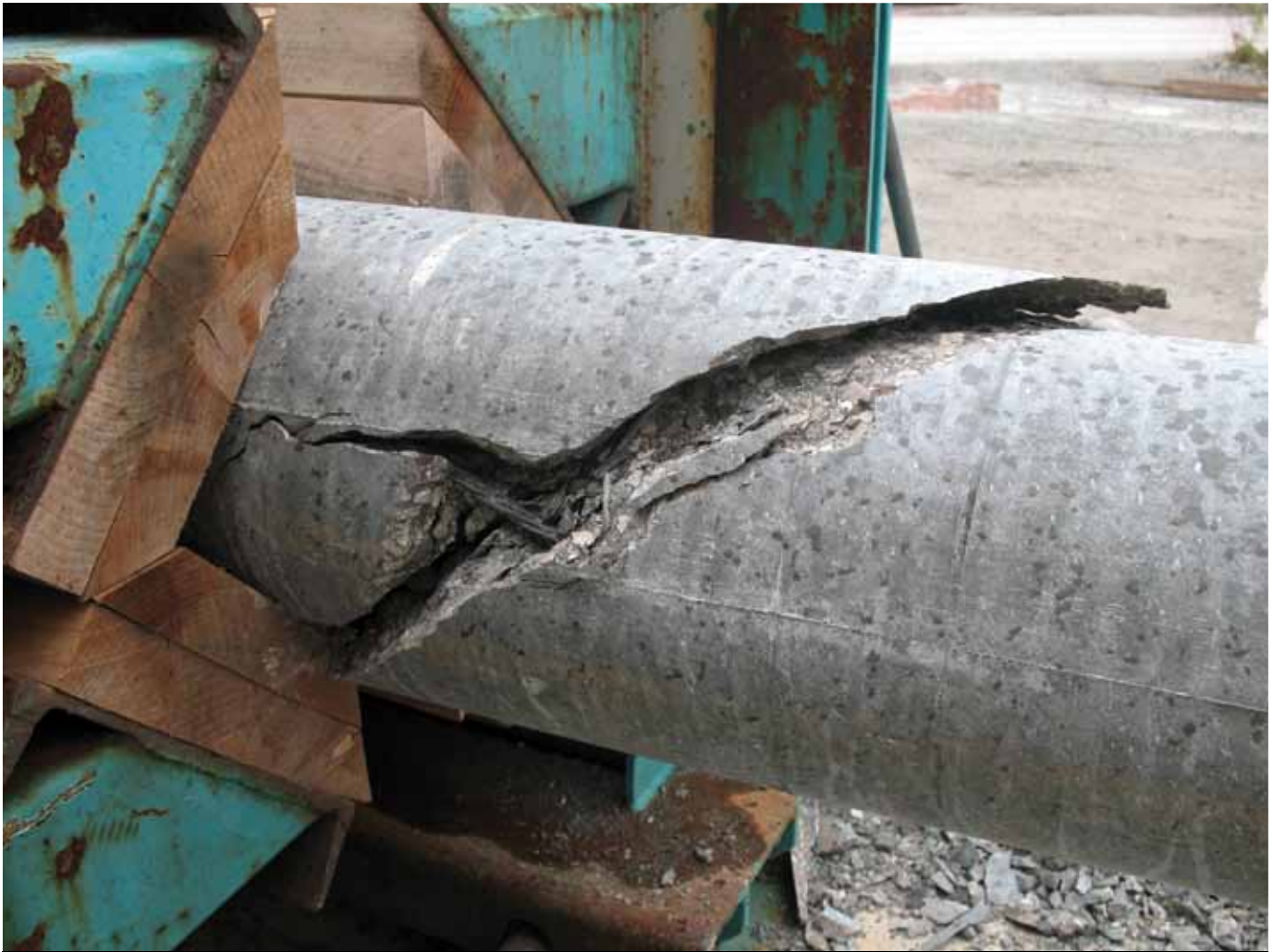
Figure 7. Typical butt clamp failure.
