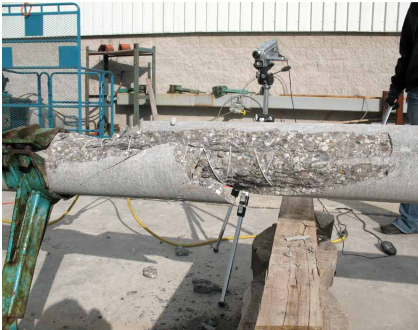
Figure 6. Typical loading collar failure.
