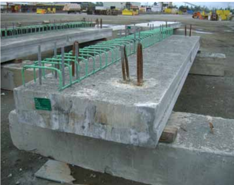
Special exterior slabs produced by Knife River Corp.—Northwest for the Volmer and Johnson Creek bridges project on US Route 26 between Portland, Ore., and the coast are cast to receive the bridge rail and match the interior slabs. Courtesy of Knife River Corp.
