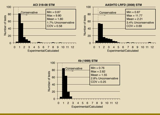
**Figure 7.** These histograms summarize the ratio of the experimental capacity over the STM estimation for all of the beams in the evaluation database (N = 179). Note: COV = coefficient of variation; N = number of test specimens that are evaluated; STM = strut-and-tie model.
