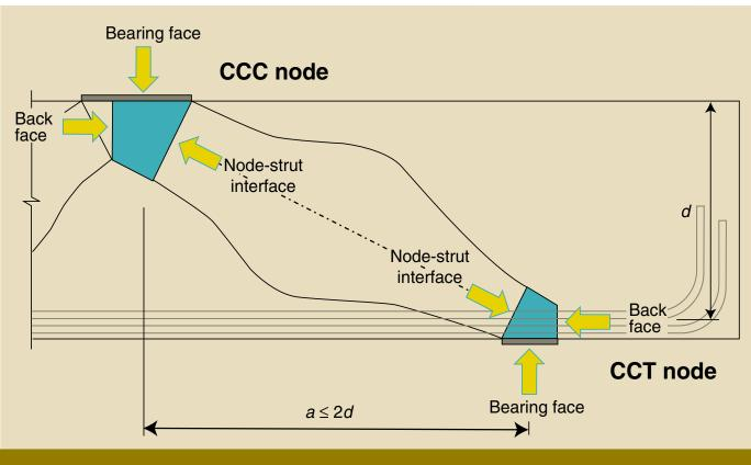
**Figure 4.** This figure shows a single-panel strut-and-tie model with nonhydrostatic nodal regions. Note: *a* = shear span; CCC = node framed by three or more intersecting struts; CCT = node framed by two or more intersecting struts and a tie; *d* = distance from extreme compression fiber to centroid of longitudinal tension reinforcement.
