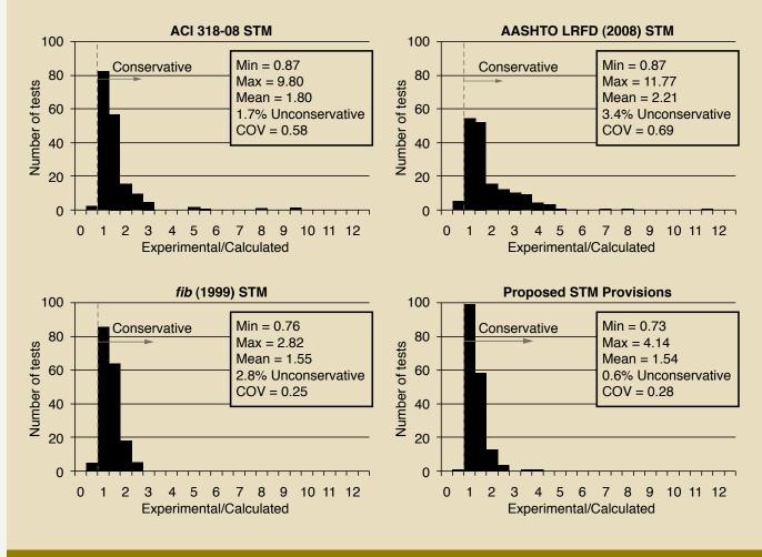
**Figure 9.** These histograms summarize the ratio of the experimental capacity over the STM estimation for all of the beams in the evaluation database. The design provisions presented in Fig. 7 are compared with the new method proposed in this paper (N = 179). Note: COV = coefficient of variation; N = number of test specimens that are evaluated; STM = strut-and-tie model.
