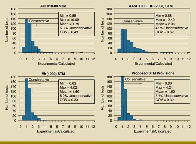
**Figure 10.** These histograms summarize the ratio of the experimental capacity over the STM estimation for all of the beams in the filtered database with  $\rho_{\perp} > 0.1\%$  (N = 382). Note: COV = coefficient of variation; N = number of test specimens that are evaluated; STM = strut-and-tie model;  $\rho_{\perp} =$  ratio of the shear reinforcement perpendicular to the plane of the strut.
