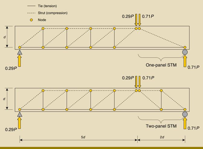
Figure 2. This figure shows both a one-panel and a two-panel strut-and-tie model that can be used to represent a deep-beam region. Note: *d* = distance from extreme compression fiber to centroid of longitudinal tension reinforcement; *P* = axial load; STM = strut-and-tie model.
