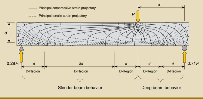
**Figure 1.** This figure shows the strain distribution in the deep and slender portion of a beam. Note: a = shear span; B region = region of a structure where the Bernoulli hypothesis is valid; d = distance from extreme compression fiber to centroid of longitudinal tension reinforcement; D region = region of discontinuity caused by abrupt changes in geometry or loading; P = axial load.
