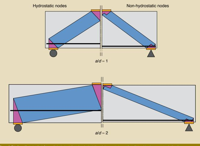
Figure 3. This figure illustrates the influence that a hydrostatic and nonhydrostatic node has on strut proportions. Note: a/d = shear span-to-depth ratio.
