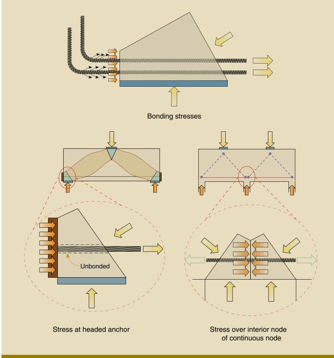
Figure 8. This figure illustrates the three different stress conditions that can occur at the back face of a CCT node. CCT = node framed by two or more intersecting struts and a tie.
