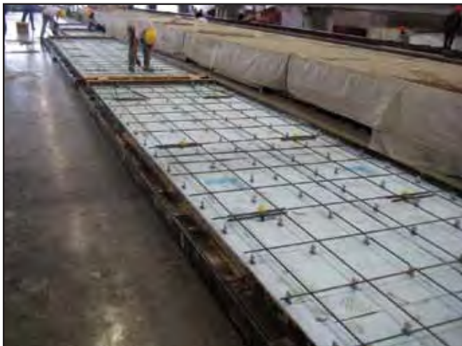
Figure 4.1.i. Pin connectors for composite action. Prestressing strand in place to prestress panel.
