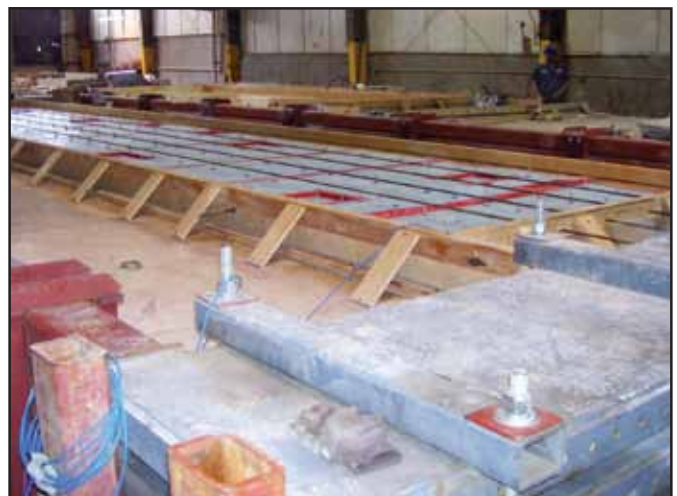
Figure 4.1.l. Prestressing strand in place to prestress panel.
