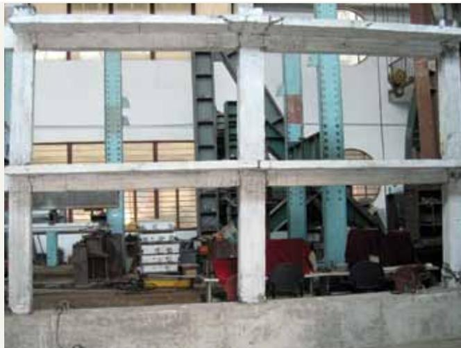
**Figure 13.** This photo shows the final failure patterns of the frame model specimen PCF-1 at the end of the test.
