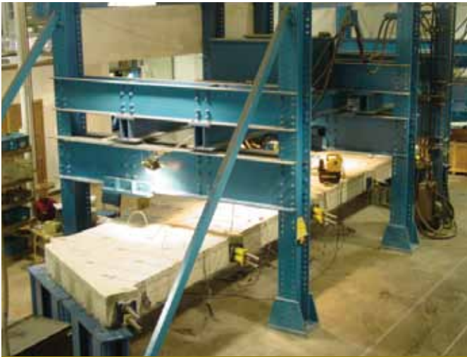
Figure 3. This photo depicts the general view of the precast, prestressed concrete box-beam bridge model.
