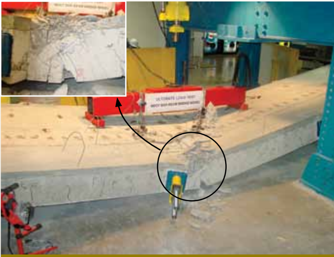
Figure 15. This photo shows the failure of the bridge model.
