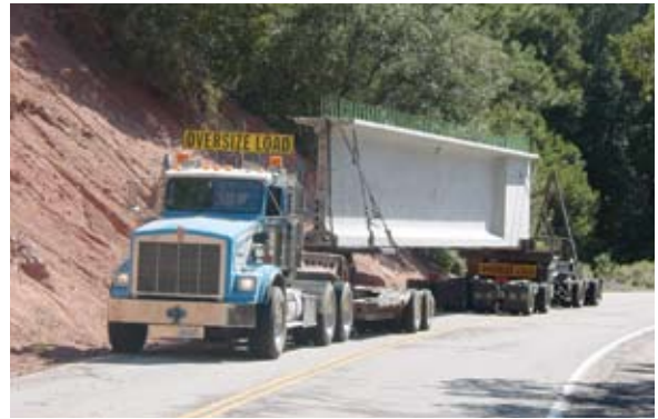
To transport the girders for the Angeles Crest Bridge No. 1 on state route 2 to the construction site, trailers were equipped with hydraulics that allowed the support on which the girder sat to be automatically adjusted for the superelevation and could maintain the girder in a vertical position. Courtesy of Pomeroy.
