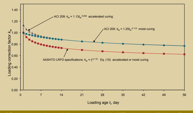
Figure 6. This graph determines the loading-age correction factor according to various methods. Note: AASHTO = American Association of State Highway and Transportation Officials; ACI = American Concrete Institute; LRFD = load- and resistance-factor design;  $t_{ie}$  = .
