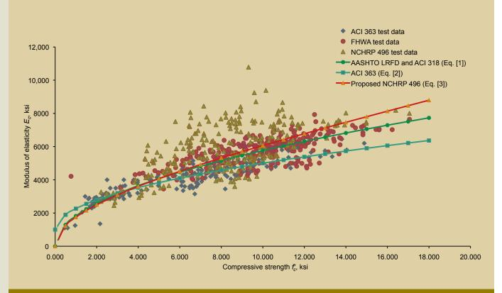
Figure 3. This graph shows the modulus of elasticity, including results of previous research. Note: AASHTO = American Association of State Highway and Transportation Officials; ACI = American Concrete Institute; FHWA = Federal Highway Administration; LRFD = load- and resistance-factor design; NCHRP = National Cooperative Highway Research Program. 1 ksi = 6.895 MPa.
