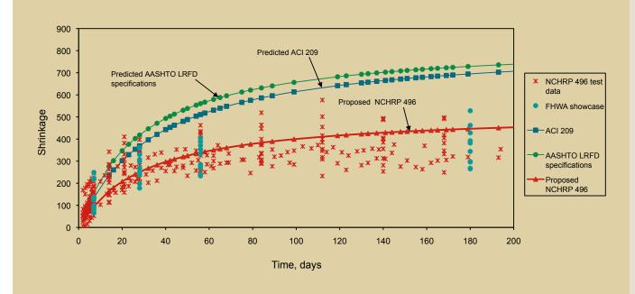
Figure 9. This graph shows the experimental results of shrinkage. Note: AASHTO = American Association of State Highway and Transportation Officials; ACI = American Concrete Institute; FHWA = Federal Highway Administration; LRFD = load- and resistance-factor design; NCHRP = National Cooperative Highway Research Program.
