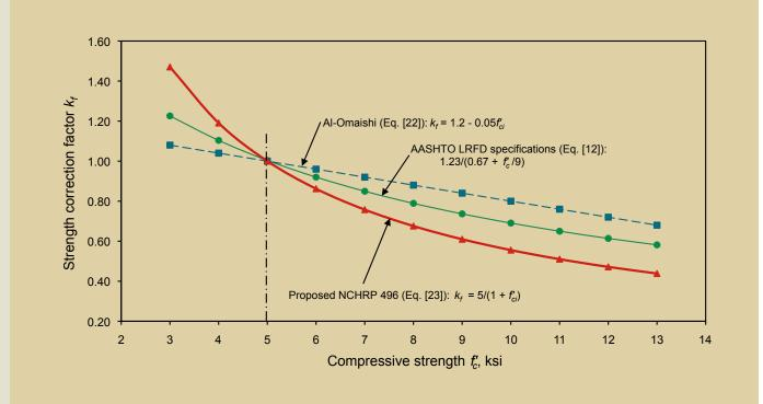
**Figure 7.** This graph shows the effect of different strength correction factors for different concrete compressive strengths. Note: Assume  $f'_{cl} = 0.8f'_{c}$ . AASHTO = American Association of State Highway and Transportation Officials;  $f'_{cl}$  = specified compressive strength of concrete at time of initial loading or prestressing; LRFD = load- and resistance-factor design; NCHRP = National Cooperative Highway Research Program. 1 ksi = 6.895 MPa.
