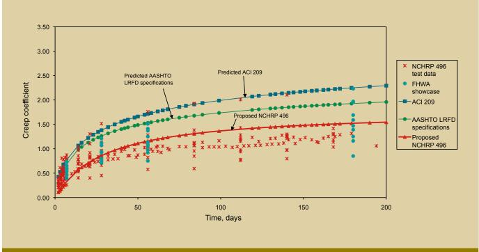
Figure 10. This graph shows the experimental results of creep. Note: AASHTO = American Association of State Highway and Transportation Officials; ACI = American Concrete Institute; FHWA = Federal Highway Administration; LRFD = load- and resistance-factor design; NCHRP = National Cooperative Highway Research Program.
