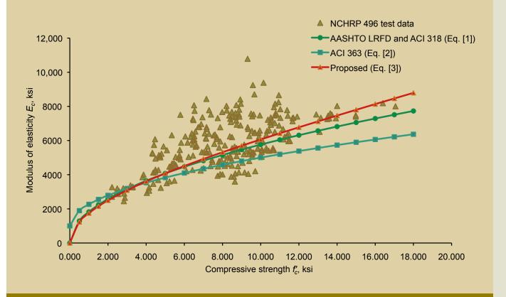
Figure 2. The modulus of elasticity was determined using results of experiments in this project. Note: AASHTO = American Association of State Highway and Transportation <u>Officials; ACI = American Concrete Institute;</u> LRFD = load- and resistance-factor design; NCHRP = National Cooperative Highway Research Program. 1 ksi = 6.895 MPa.
