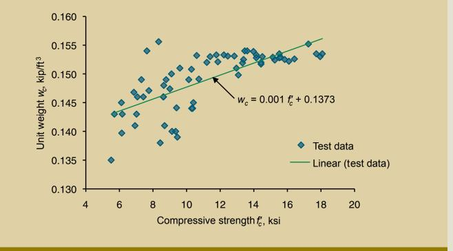
Figure 1. This graph shows the relationship between the density and compressive strength of concrete. Note: 1 ksi = 6.895 MPa; 1 kip/ft<sup>3</sup> = 0.016 kg/m<sup>3</sup>.
