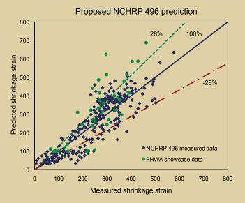
Figure 11. This graph compares measured with predicted values of shrinkage strain using AASHTO LRFD specifications, the ACI 209 committee report, and the proposed NCHRP 496 methods. Note: AASHTO = American Association of State Highway and Transportation Officials; ACI = American Concrete Institute; FHWA = Federal Highway Administration; LRFD = Ioad- and resistance-factor design; NCHRP = National Cooperative Highway Research Program.
