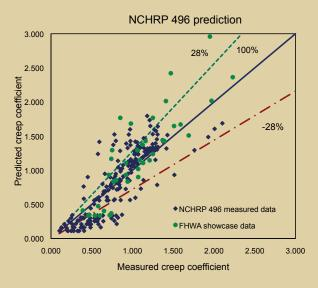
Figure 12. This graph compares measured with predicted values of creep coefficient using AASHTO LRFD specifications, the ACI 209 committee report, and proposed NCHRP 496 methods. Note: AASHTO = American Association of State Highway and Transportation Officials; ACI = American Concrete Institute; FHWA = Federal Highway Administration; LRFD = load- and resistance-factor design; NCHRP = National Cooperative Highway Research Program.
