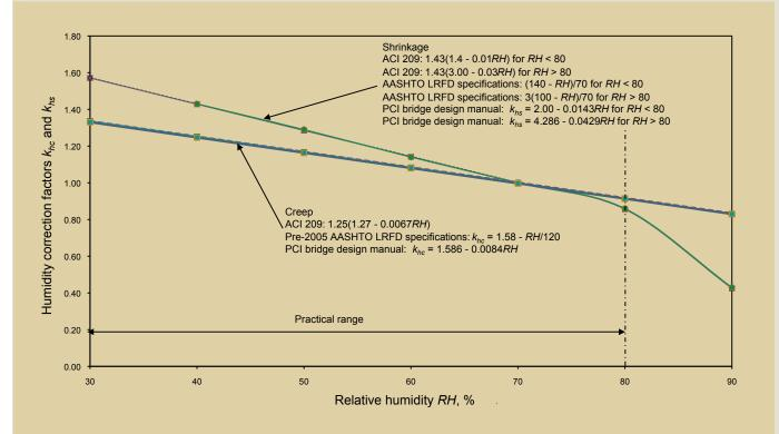
Figure 4. This graph determines the humidity correction factor according to various prediction methods. Note: Values predicted by various methods are normalized to unity at a humidity of 70%. AASHTO = American Association of State Highway and Transportation Officials; ACI = American Concrete Institute; LRFD = load- and resistance-factor design.
