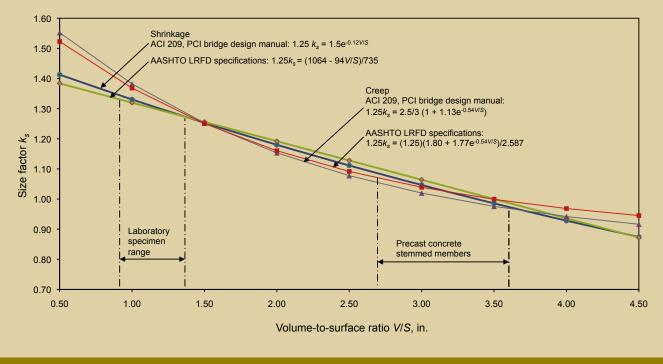
Figure 5. This graph determines the size correction factor according to various methods. Note: AASHTO = American Association of State Highway and Transportation Officials; ACI = American Concrete Institute; LRFD = load- and resistance-factor design. 1 in. = 25.4 mm.
