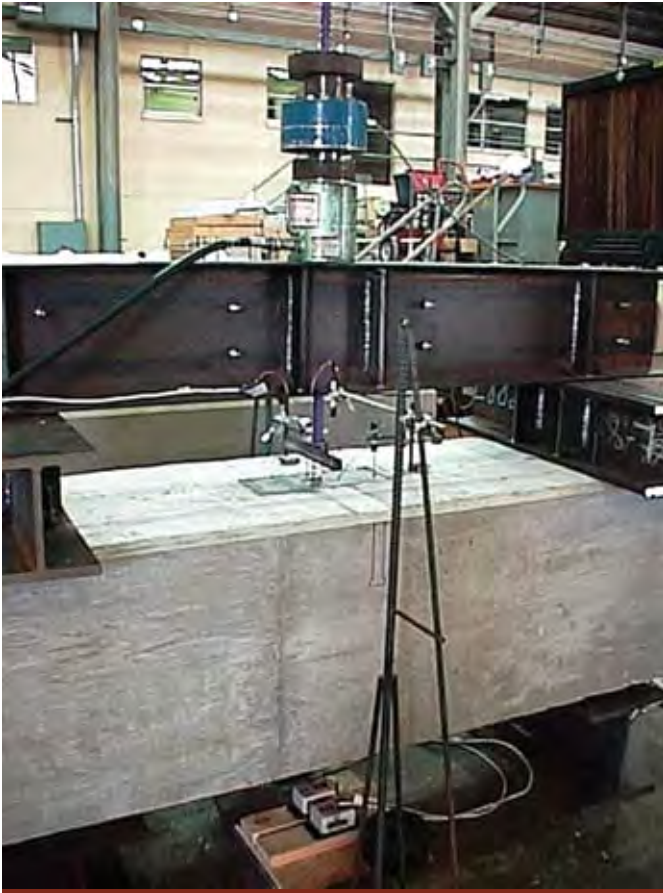
Figure 8. This test setup is for grout-pocket and grouted-duct tension pullout tests.
