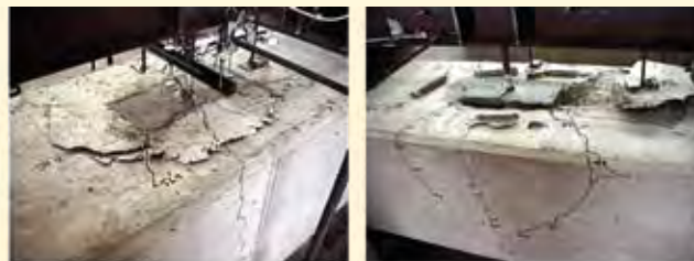
Straight reinforcing bar SL13 Headed reinforcing bar SL03
