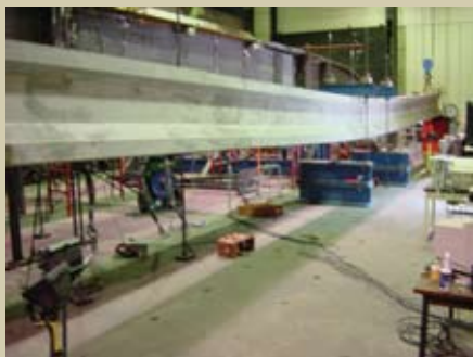
Testing at the Federal Highway Administration laboratory in McLean, Va., on a 24-m-long (80 ft), ultra-high-performance concrete American Association of State Highway and Transportation Officials Type II girder deflecting at 480 mm (19 in.) illustrates the ductility of this material under loading. Photo courtesy of Lafarge Canada Inc.
