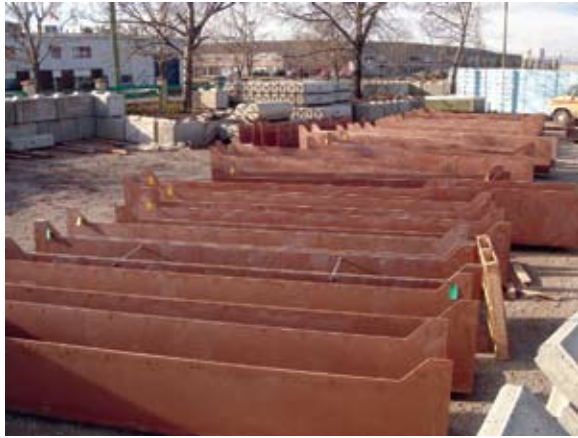
Ultra-high-performance fiber-reinforced precast concrete troughs are ready for transport at the Lafarge precasting facility. Photo courtesy of Lafarge Canada Inc.
