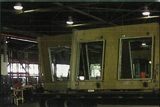
Fig. 27. Coordination between the precaster and the glazier resulted in cost savings and schedule acceleration.
