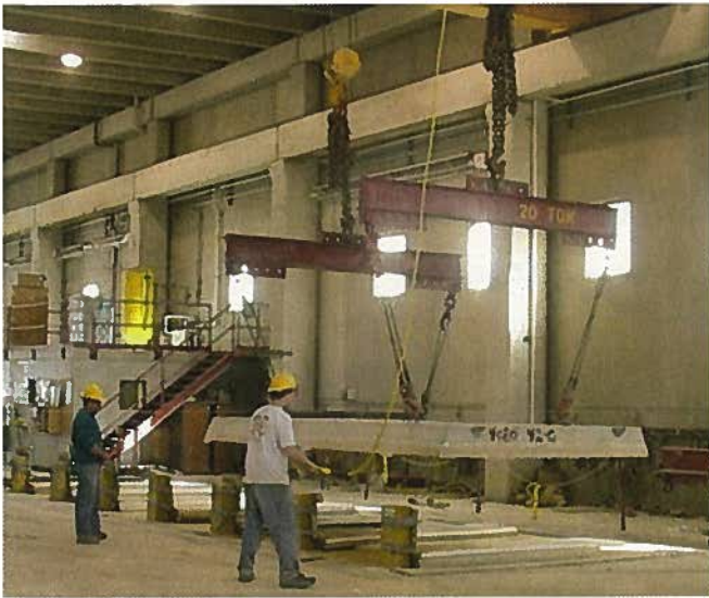
Fig. 7. Precast concrete manufacture involves considerable handling and moving of both materials and finished products, creating ample opportunities for reducing transport and waiting waste.
