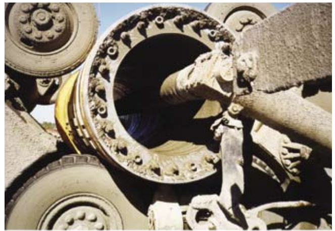
Fig. 15. Manufacture of spun-cast cylindrical piles at Gulf Coast Pre-Stress, Inc. facilities.
