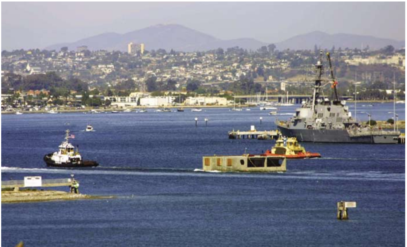
Fig. 1. Floating precast concrete modular pier test bed on a 1770 km (1100 mile) open-ocean transport to its final destination at a naval base in San Diego, California, September 2004. (U.S. Navy photo. Photographer: Erick Huang.)
