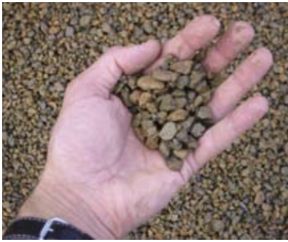
Fig. 10. Manufactured lightweight aggregate was used in a durable concrete mix that attained an average compressive strength of more than 50 MPa (7.5 ksi) after 56 days.
