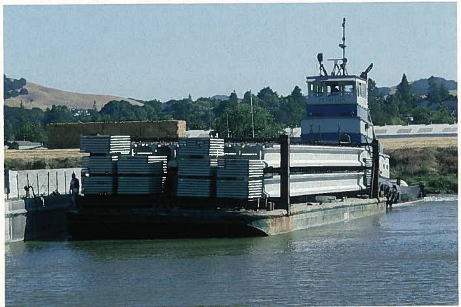
Fig. 21. At the precast plant boat slip, one of the loaded barges prepares for its 60 mile (100 km) southbound trip down the Petaluma River to the San Francisco Bay and the bridge site. (Courtesy of CALTRANS District 4 Photography Department)
