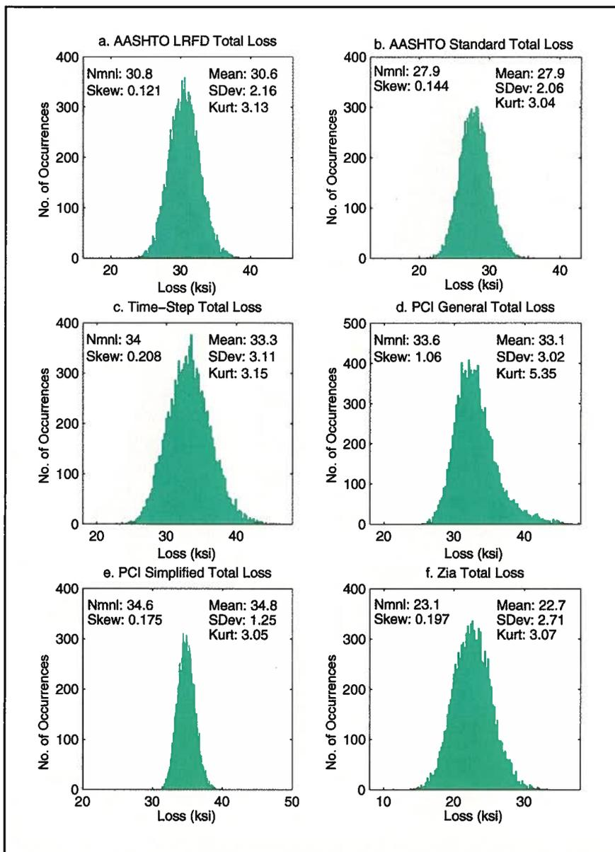
Fig. 5. Monte Carlo Simulation output distributions showing total prestress losses for all methods (box beam example).
