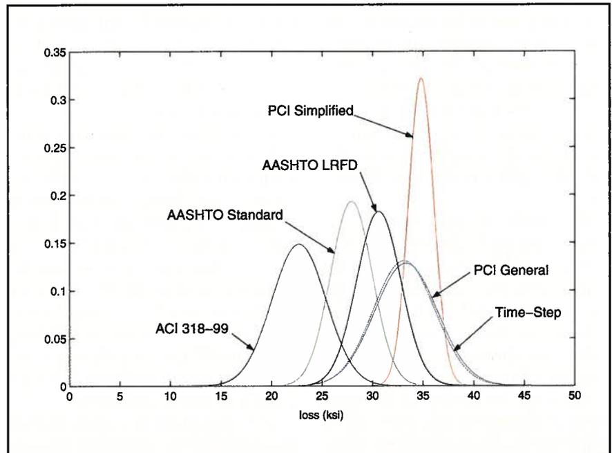
Fig. 7. Total prestress losses for all methods (box beam example).
