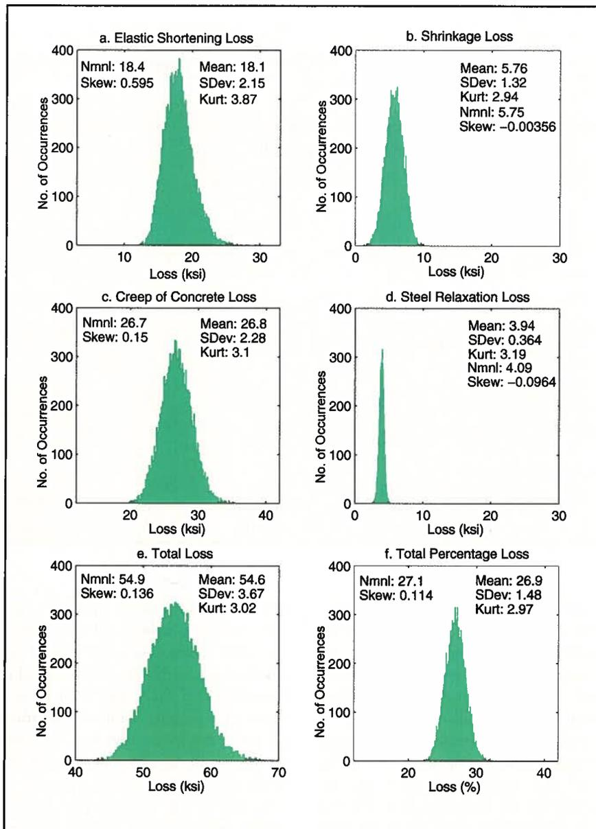
Fig. 3. Monte Carlo Simulation output distributions using AASHTO LRFD individual loss components for I-beam example.
