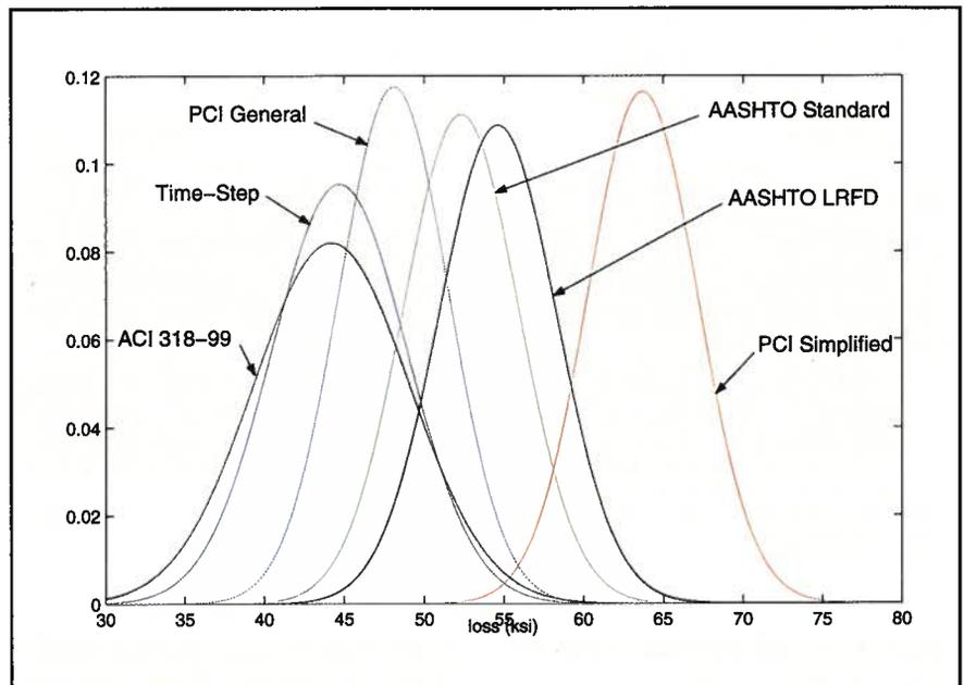
Fig. 6. Total prestress losses for all methods (I-beam example).
