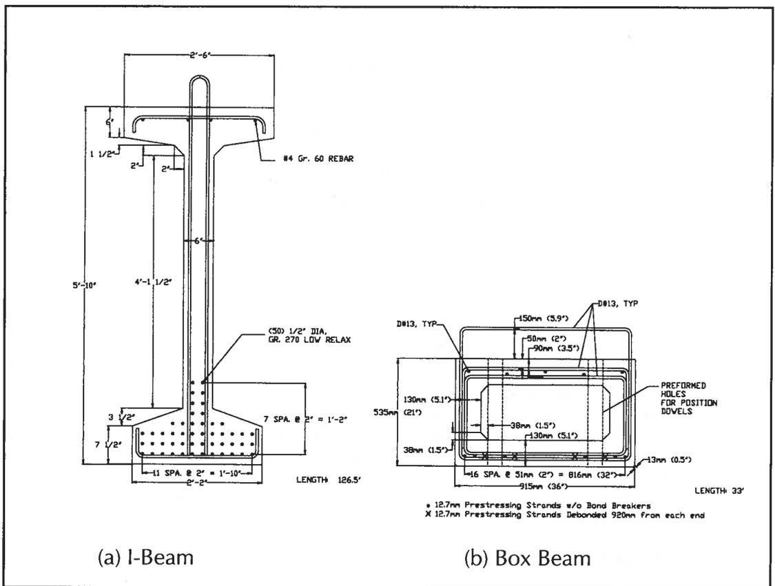
Fig. 1. Cross sections of beams considered showing dimensions and reinforcing details.
