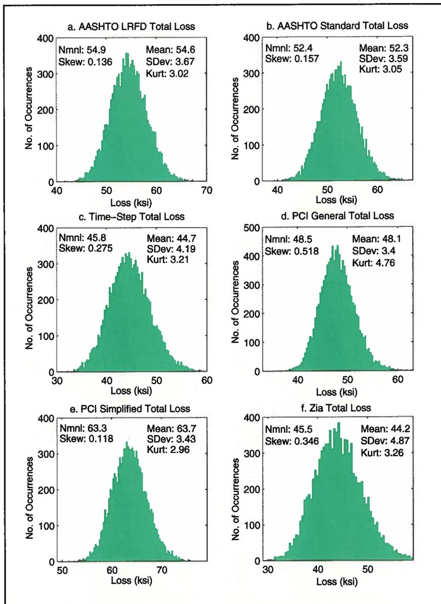
Fig. 4. Monte Carlo Simulation output distributions showing total prestress losses for all methods (I-beam example).
