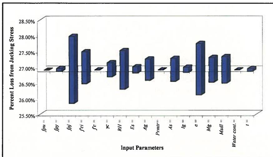
Fig. 2. Parametric study results using AASHTO LRFD method for I-beam example.
