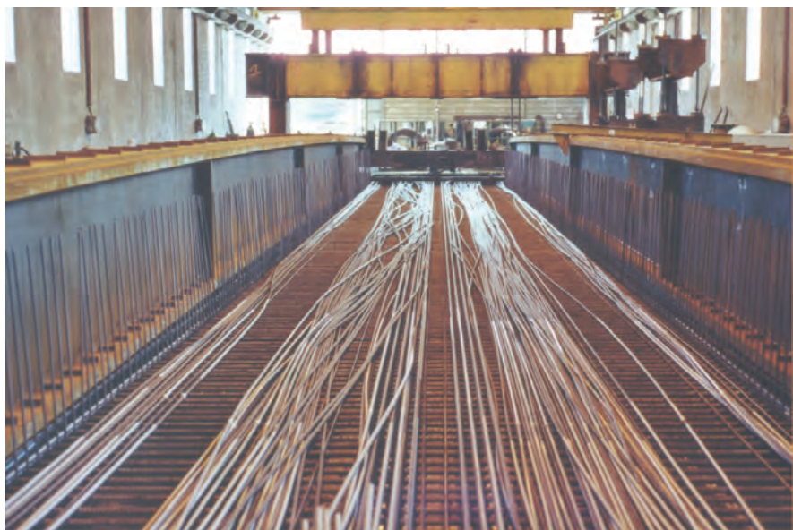
Fig. 14. Precambered (preflexion) stage of steel beams showing prestressing tendons and reinforcing steel in plant. (Photograph by Bernard Espion)
