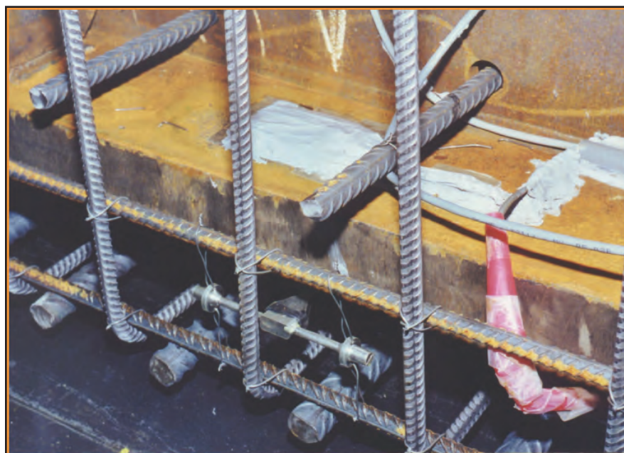
Fig. 35. Bridge deck instrumented with strain gauges. (Photograph by Bernard Espion)
