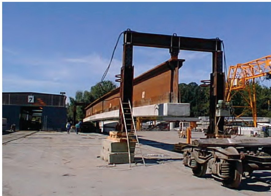
Fig. 3. Flexstress (precambered) beam at precasting yard. (Courtesy of Ronveaux Company)
