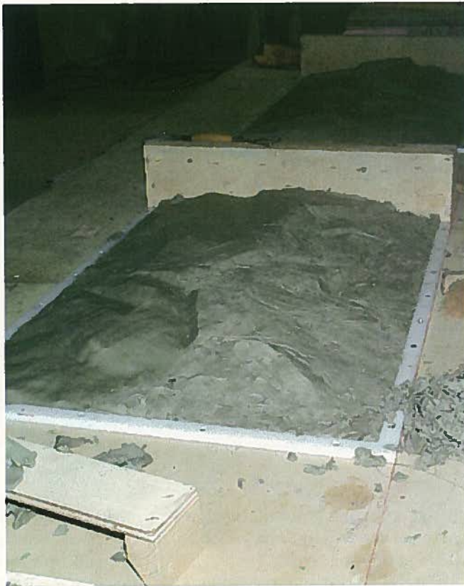
Fig. 9. Clay forms were hand-sculpted into diverse cut-stone patterns and variations at Rocky Mountain Prestress to simulate the Texas Pearl granite of the Liberty Media Corporate Headquarters.
