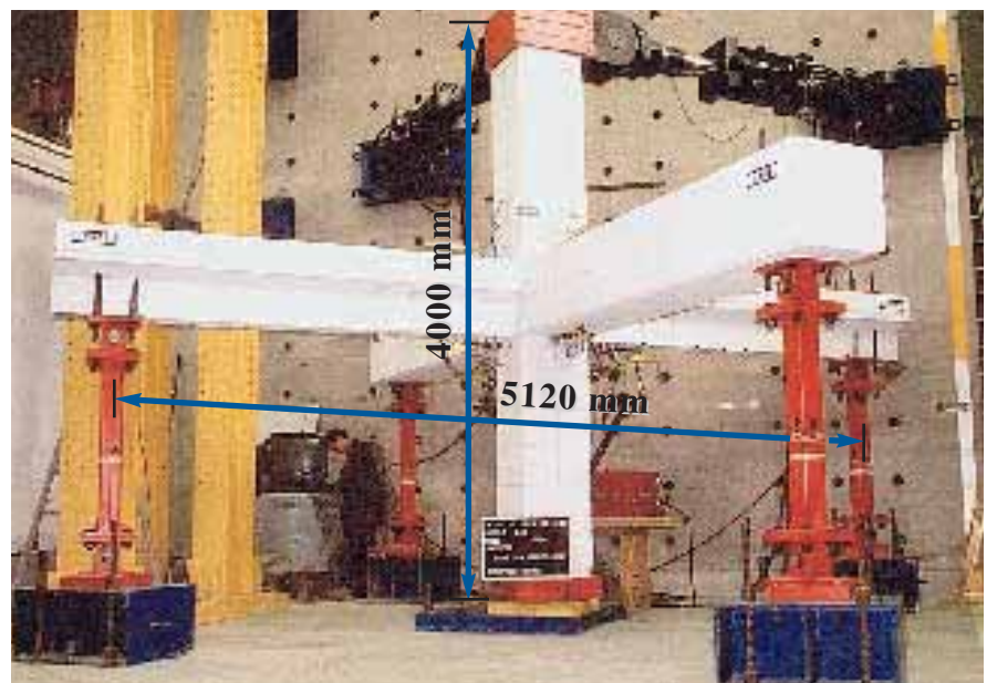
Fig. 2. Specimen geometry and testing rig.
