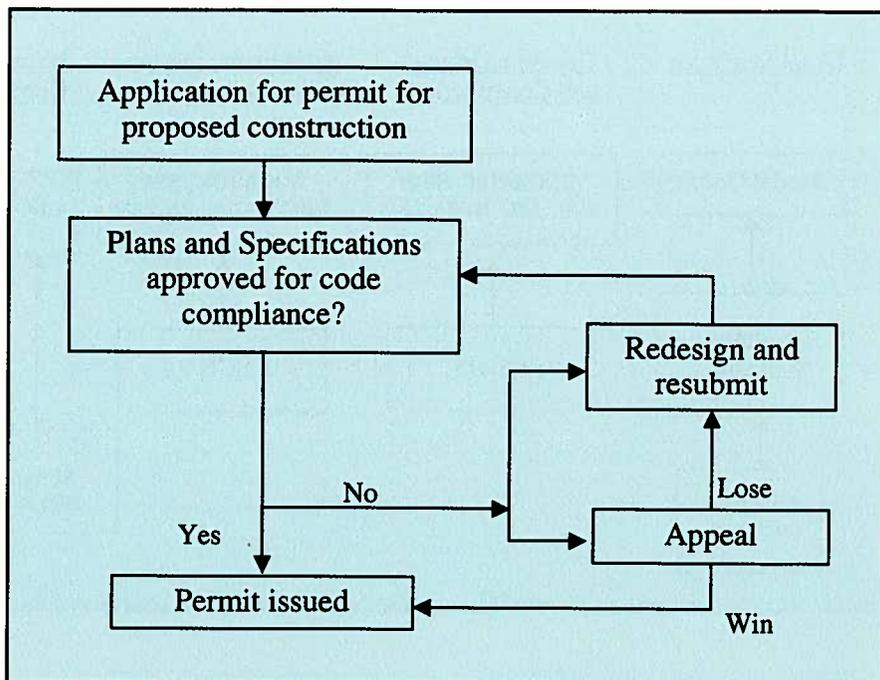
Fig. 1a. Issuance of construction permit.
