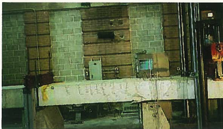
Fig. 13. Overview and closeup of typical failure due to crushing of concrete for cantilever specimens.
