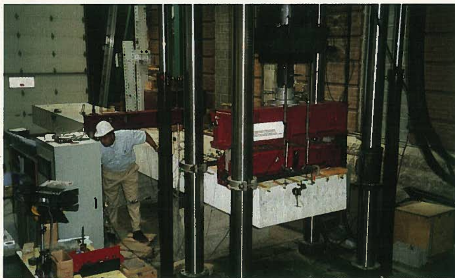
Fig. 8b. Testing of cantilever specimens in laboratory.
