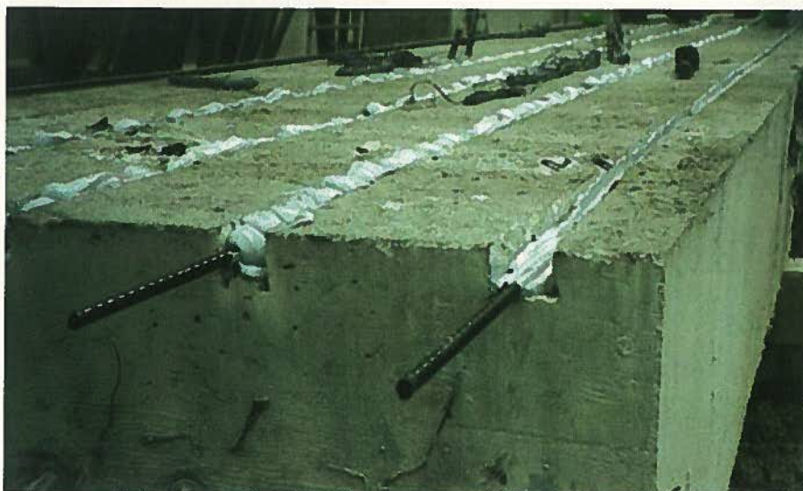
Fig. 4. CFRP bars inserted in epoxy.
