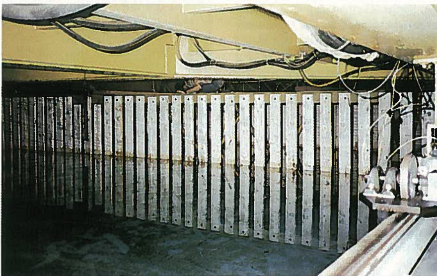
Fig. 11. Model of downwave breakwater elements at low tide in wave tank.
