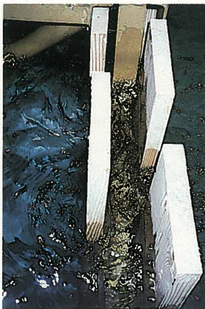
Fig. 10. Plan of model breakwater elements in wave tank.
