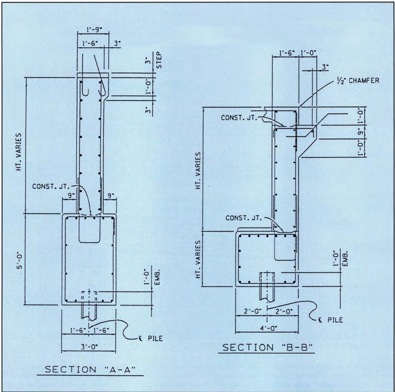
Fig. 6. Sections of integral abutment of bridge (see also Fig. 5).
