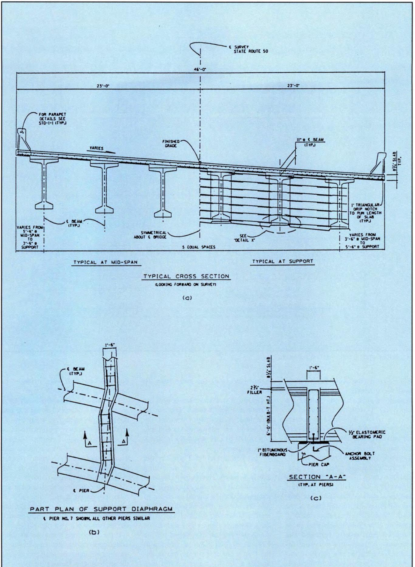
Fig. 3. Typical cross section of bridge at midspan and support together with partial plan and section of support diaphragm.
