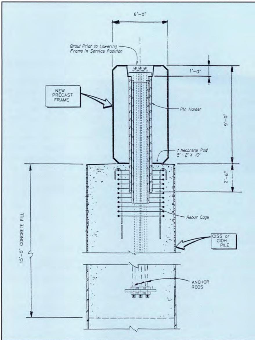
Fig. 2. Typical section showing precast frame-to-pile connection.
