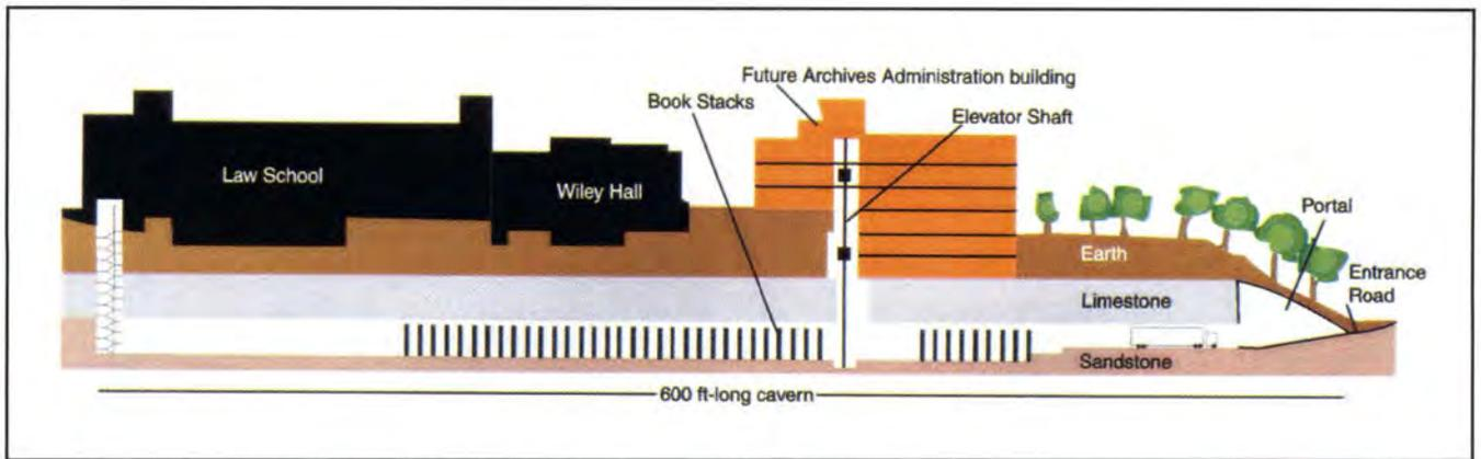
Fig. 1. Section view of library access center showing cavern, existing buildings and new construction.
