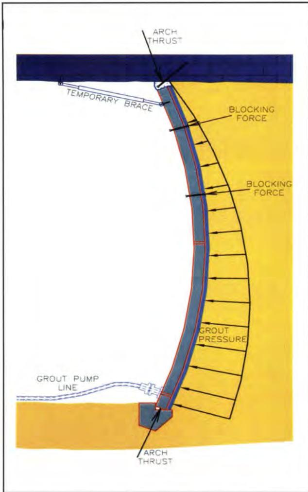
Fig. 3. Force diagram showing curved panel interaction.
