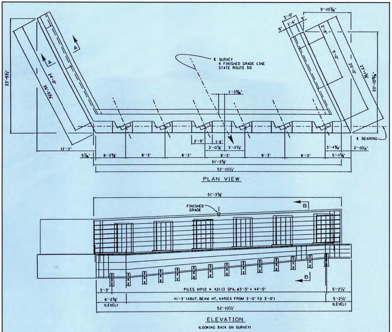
Fig. 5. Plan and elevation of integral abutment of bridge (see also Fig. 6).
