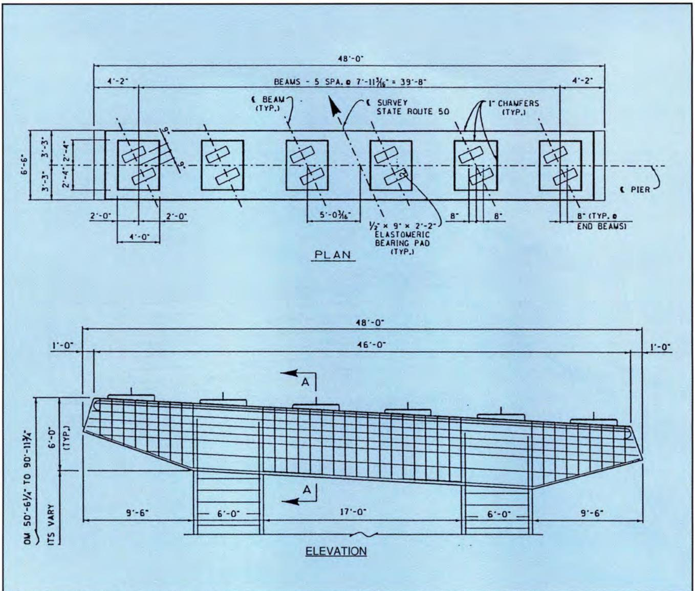
Fig. 4. Plan and elevation of column bents.
