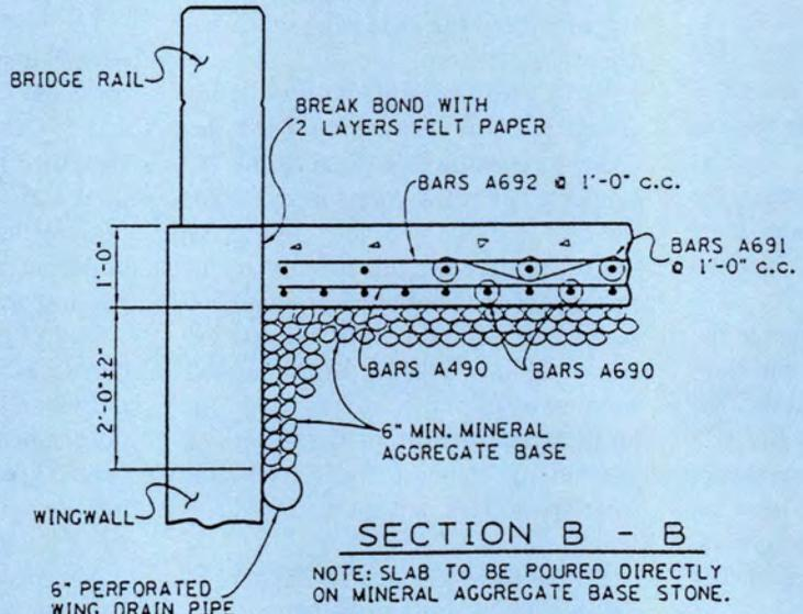
Fig. 8. Plan and section of approach roadway pavements (see also Fig. 9).
