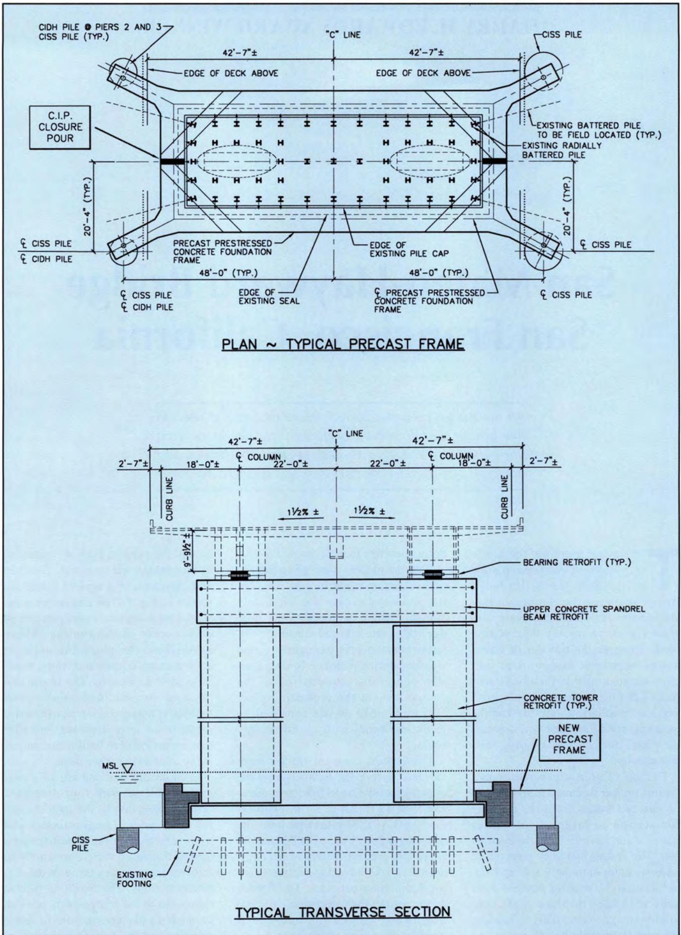
Fig. 1. Typical plan and elevation of precast frame unit.
