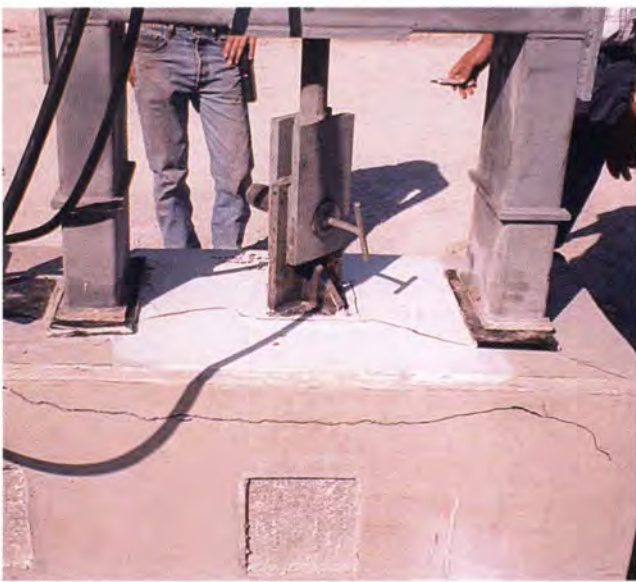
(a) Cracking pattern at concrete failure.
