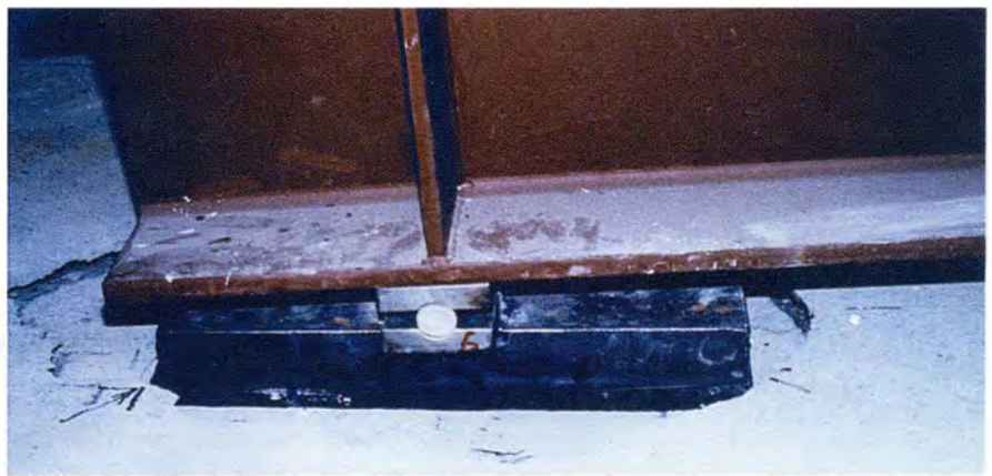
Fig. 16. Punching shear failure of panel.
