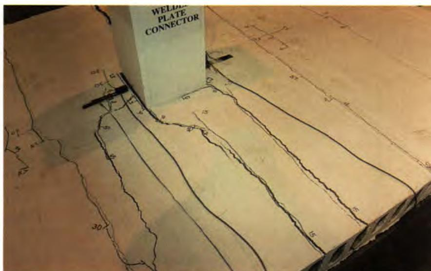
Fig. 10. Transverse cracking in floor slab at ultimate moment in Test TW1 by Gorgun (Ref. 20).
