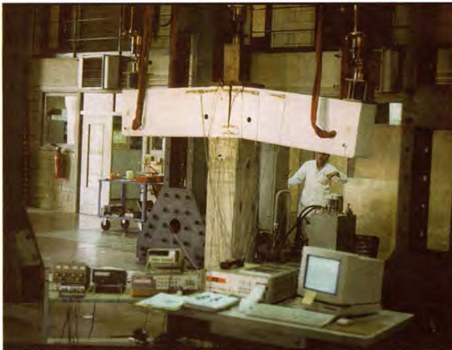
Fig. 13. Test arrangement to study beam-to-column head connections at CERIB (Refs. 13 and 14) (Courtesy: CERIB, Epernon, France).
