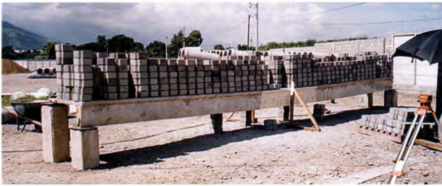
Fig. 20. Load testing of single riser specimen.
