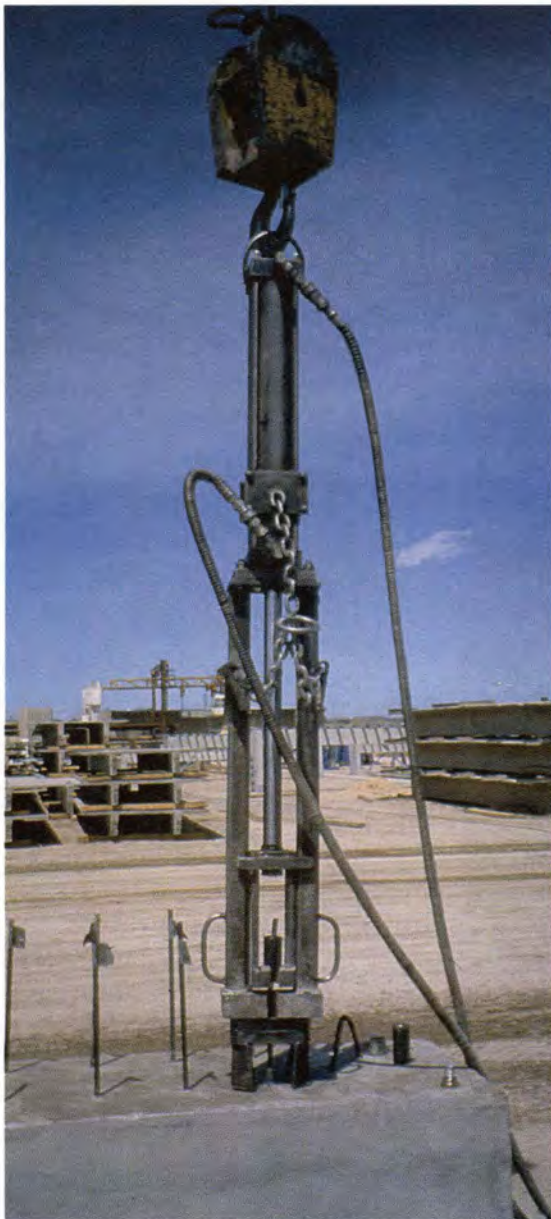
Fig. 15. Pull-out load applied with single strand jack (preliminary pull-out test series).
