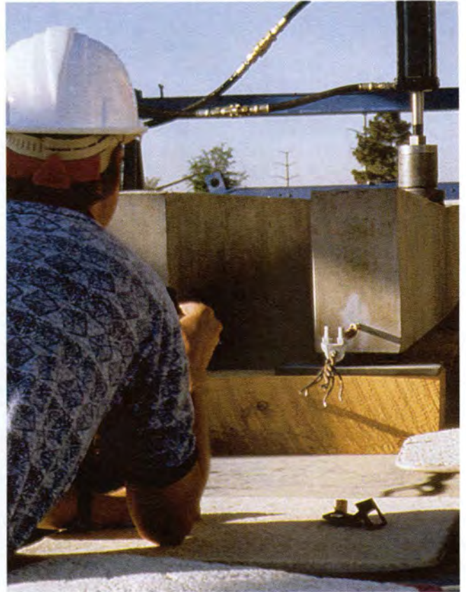
Fig. 26. Beam TW-5 (north end) approaching failure, deflection = 2 in. (51 mm). Observing end for strand slip during loading (June 8, 1996).
