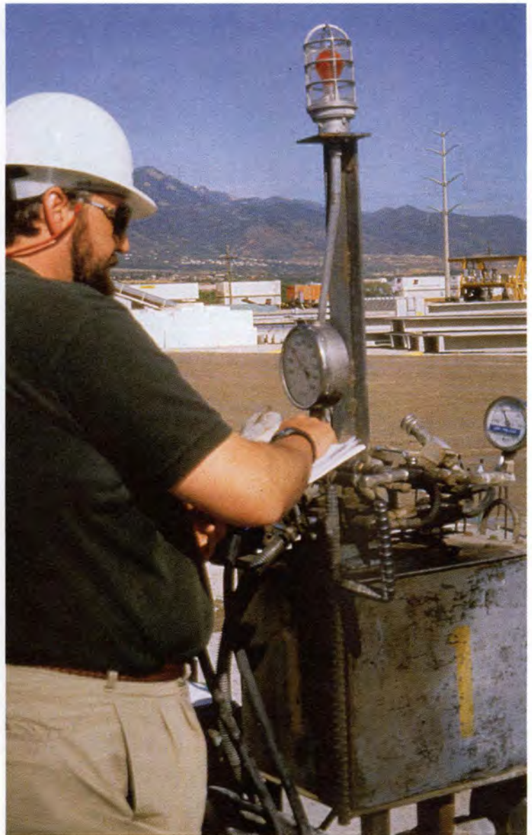
Fig. 16. Advisory group member Bruce Russell applying load at 20 kips per minute (89 kN/minute) and recording maximum pull-out load (May 18, 1996).
