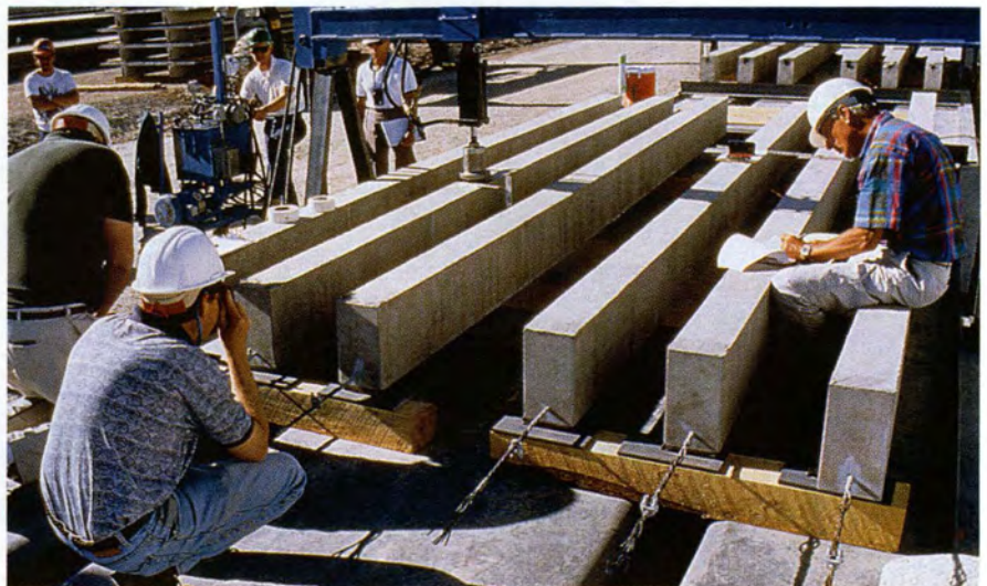
Fig. 24. First six-beam line at start of development length test. Simple span, L_e = 6.08 \text{ ft} (1.85 m) (June 8, 1996).
