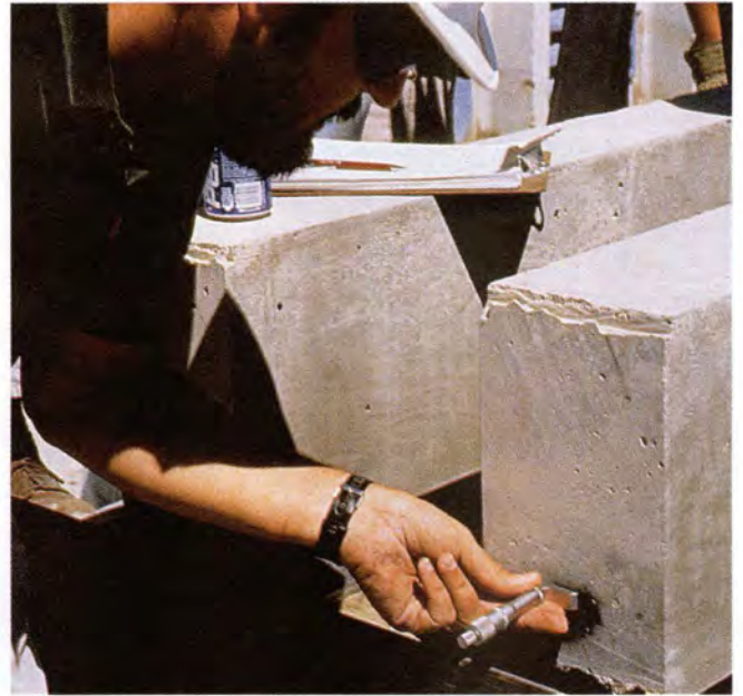
Fig. 21. Measurement of initial strand slip at release of prestress, saw-cut end, June 7, 1996 (similar at May 18, 1996).
