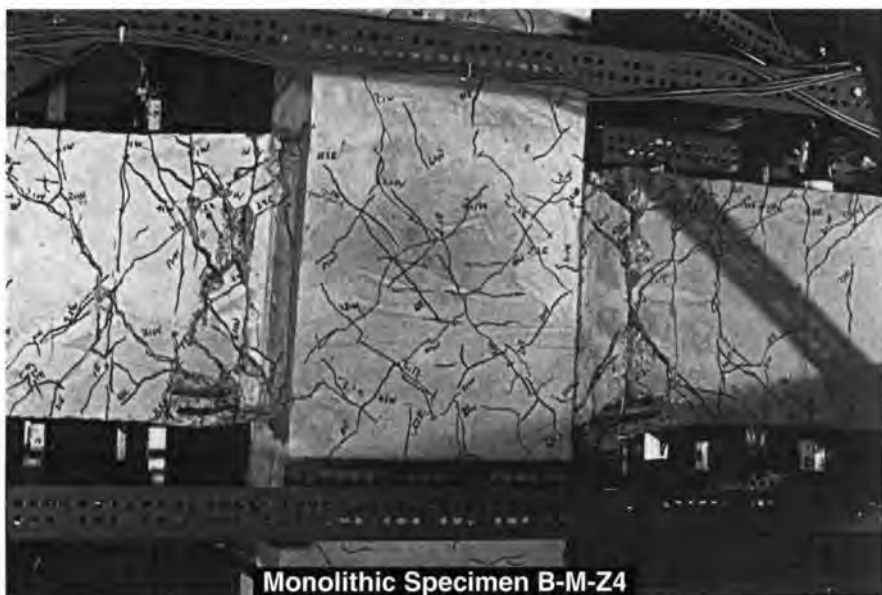
Fig. 9. Precast (top) and monolithic (bottom) specimens at failure.
